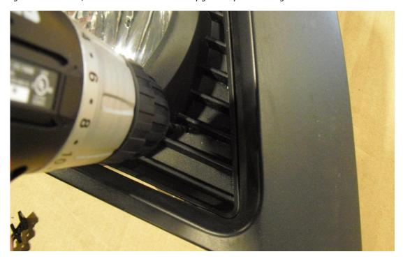
6. Once your holes are drilled, use the supplied hardware and attach outer pieces as shown with a phillips-headed screwdriver and 6mm socket.
