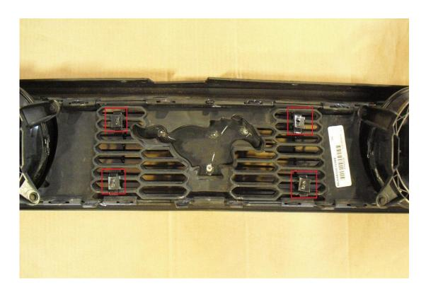
5. Place the outer pieces of your billet grille overlay over the factory grille and mark where you will have to drill a small hole for the mounting hardware. Outer pieces are side-specific, so make sure they are on the correct side before marking. Use a drill and 9/64 bit to drill holes in the factory grille for your mounting hardware.
