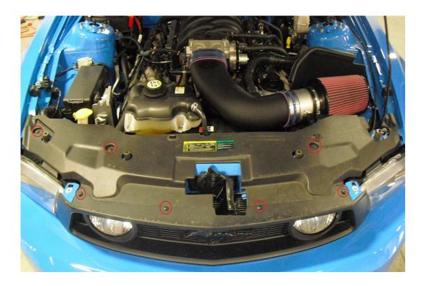
2. Remove two upper headlight mounting bolts (10mm), and two upper bumper cover mounting bolts (8mm).
