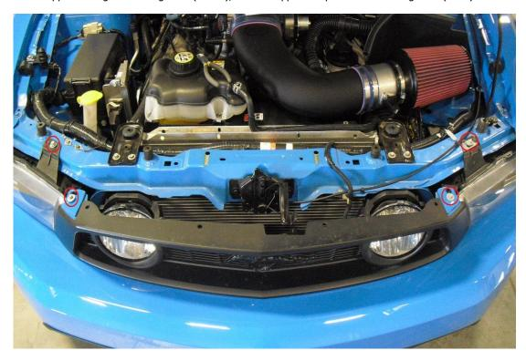
3. Use a flat-headed screwdriver to carefully pry the four outermost mounting tabs of the grille (two on each side) from the bumper cover. Once these outer tabs are loose, carefully but firmly pull up and out on the grille to fully release it from the bumper cover. Make sure to unplug the fog light wiring harnesses before completely removing the grille from the vehicle if it is so equipped.
