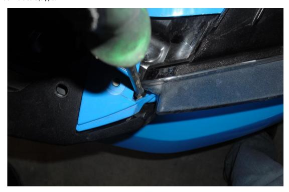
The below photo shows the mounting points of the grille to the front bumper cover:
