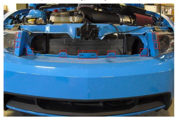
4. Install the billet overlay by placing it over the factory plastic grille and using the supplied hardware to attach it as shown. If your Mustang is a V6, there will be three mounting points, one at the top and two on the bottom. If your car is a GT, it will mount as shown with four mounting points in the center section of the grille.
