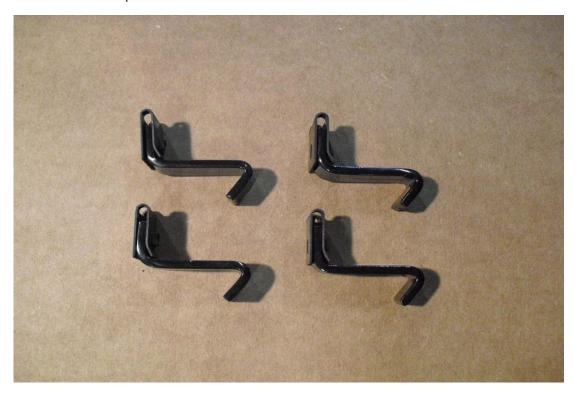
3. Pre-thread the hardware on the grille using the four U-Clip / J-Hook assemblies from Step 3 and the four included sheet metal screws. Do not fully tighten the screws, only thread them in 3-4 turns.
