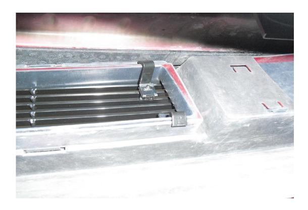
5. Once all of the hooks are secured around the factory bumper, use a Phillips head screwdriver to tighten the screws from the front of the vehicle.
