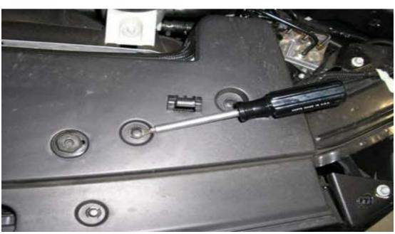
2. Remove the shroud to gain access to the back of the factory grille.
