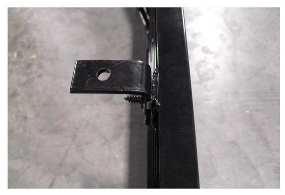
10. Complete installation of billet grille by using the final six supplied screws to secure it to the bracket you have installed in previous steps. When grille is properly aligned, fully tighten all screws on grille as well as the two screws holding the long L tabs to the upper radiator support. When grille is secure, reinstall the factory radiator cover using the six push tabs you removed in Step 1.
