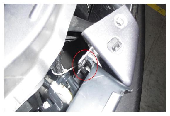
3. Before the grille is completely removed from the vehicle, make sure to unplug the fog light harnesses and securely tie them to the radiator support so they do not make contact with the radiator itself.
