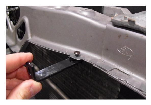
8. Place two U nuts onto the slotted portions of the long L tabs. Using the supplied screws, mount the long L tabs in the holes vacated by the fasteners you removed in Step 7. Do not fully tighten the screws as you may need to adjust them during final installation of the grille. Install the removed fasteners into the provided holes in the long L tabs.
