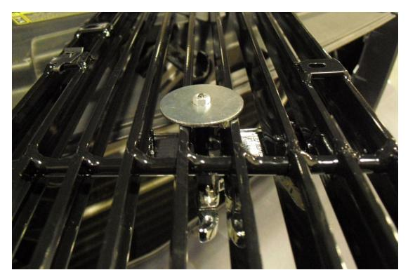
5. Place four of the supplied U nuts onto the 90 degree side of the four supplied U tabs and insert them into the tabs of the front fascia as shown. (Note: Narrow U tabs must be placed on the outside tabs)
