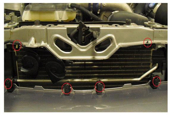
9. Place two U nuts onto the slotted portions of the short L tabs. Using supplied screws, mount the short L tabs to the inner holes of the grille as shown below. These will be used to reinstall your plastic factory radiator cover.
