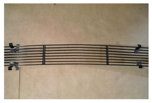
4. Place the billet grille over the factory grille. From underneath the car, adjust the J-Hooks to wrap around the factory plastic grille as shown.
