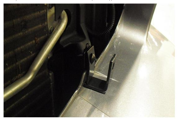
7. Place four U nuts onto outside of U tabs installed in Step 5. Remove two plastic fasteners from front radiator support, one holds a wiring harness and the other holds the hood release cable
