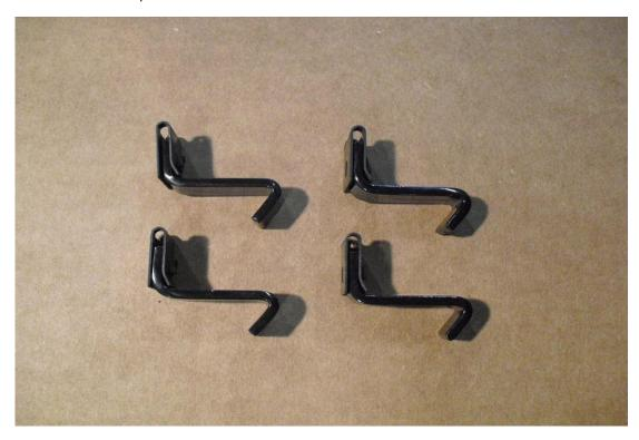
3. Pre-thread the hardware on the grille using the four U-Clip / J-Hook assemblies from Step 3 and the four included sheet metal screws. Do not fully tighten the screws, only thread them in 3-4 turns.
