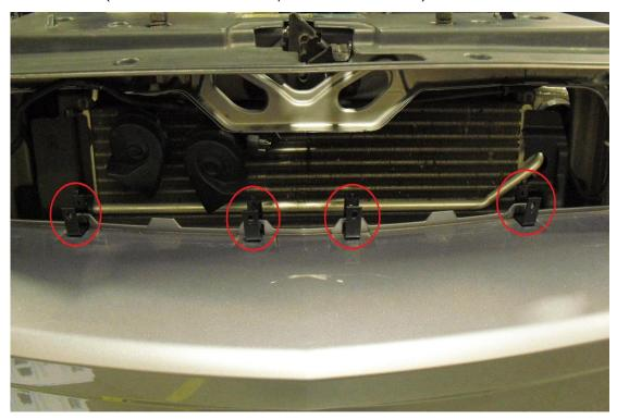
6. Install a clamp tab onto each of the U tabs and secure to bumper with supplied screws as shown.
