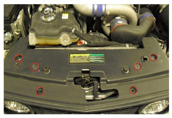
2. Remove the factory upper grille by pulling firmly and releasing it from the eight tabs that hold it to the front fascia. There are two on either side of the grille and four on the bottom lip.
