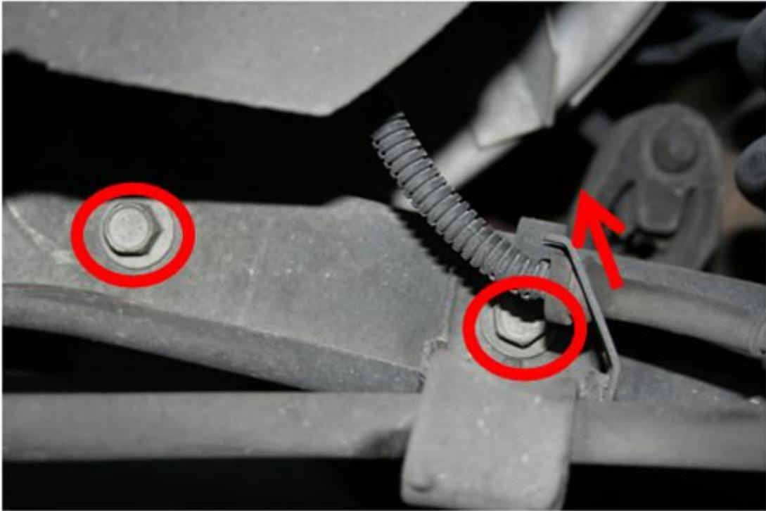
4. I did this on both sides of the vehicle and moved the sway out of the way. If you were planning on replacing your sway bar now would be a good time to do so.
