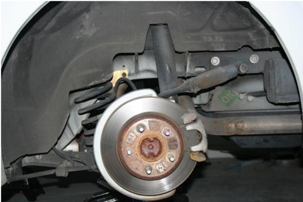
3. Next you will need to remove the harness from the bracket. Then remove the bolts with a 13mm socket and ratchet wrench. These bolts are what connect the sway bar to the control arm and are identical on both sides.
