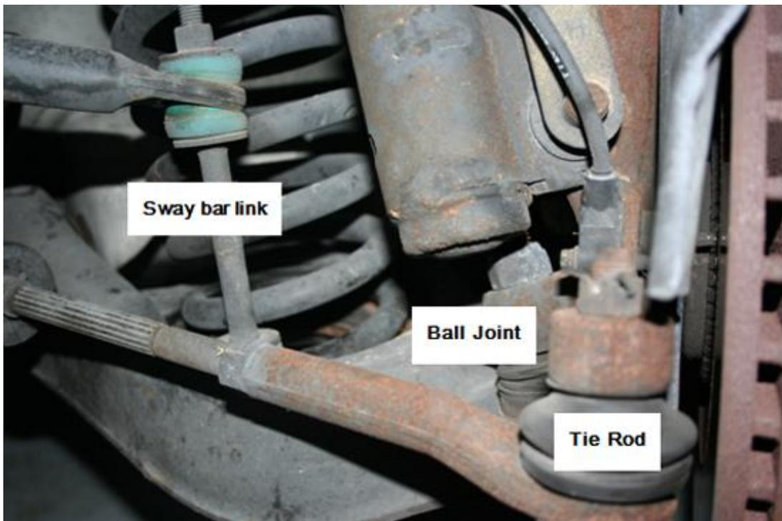
11. First remove the nut from the sway bar link underneath the control arm with a 15mm deep well socket.
