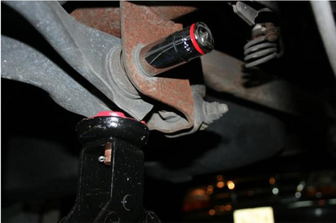
6. With the bolt removed slowly lower the jack down to release the tension on the spring. You should be able to move the spring. If not, reassemble the control arm and jack the vehicle up higher.
