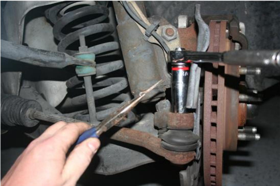
13. Now use a pry bar to apply slight pressure to the tie rod end. Then hit the spindle with a mallet and the tie rod end should come free. Now complete the removal of the castle nut to free the tie rod from the spindle.
