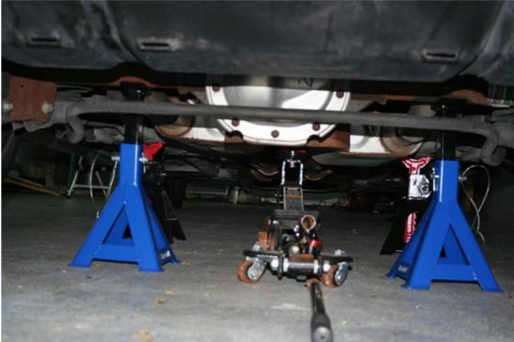
2. Remove the tires from the rear of the vehicle with a 13/16 socket and ratchet wrench or tire iron. This is done to gain access to the sway bar bolts and the control arm bolts.
