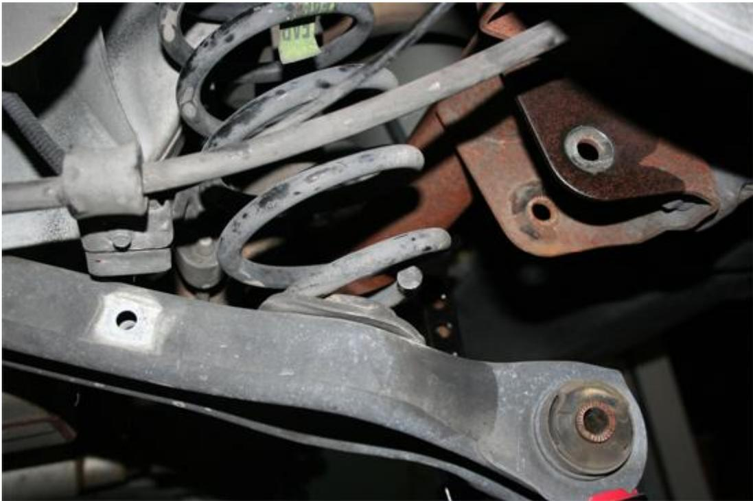
7. Now remove the old spring and place the isolator on to the new spring.
