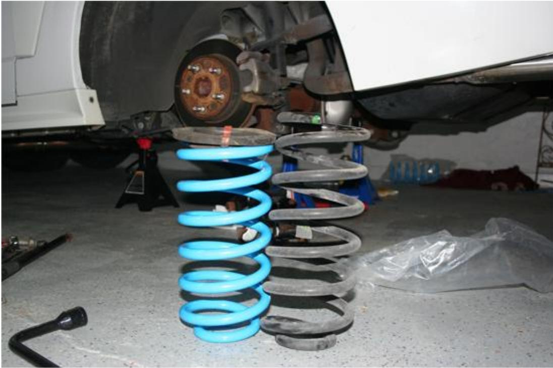
8. Insert the new spring and ensure that where the spring is cut on the bottom is facing toward the driver's side of the vehicle. Jack the control arm back up into place and bolt it back together. Repeat for the other side with the same instructions and then reinstall the sway bar and tires.
