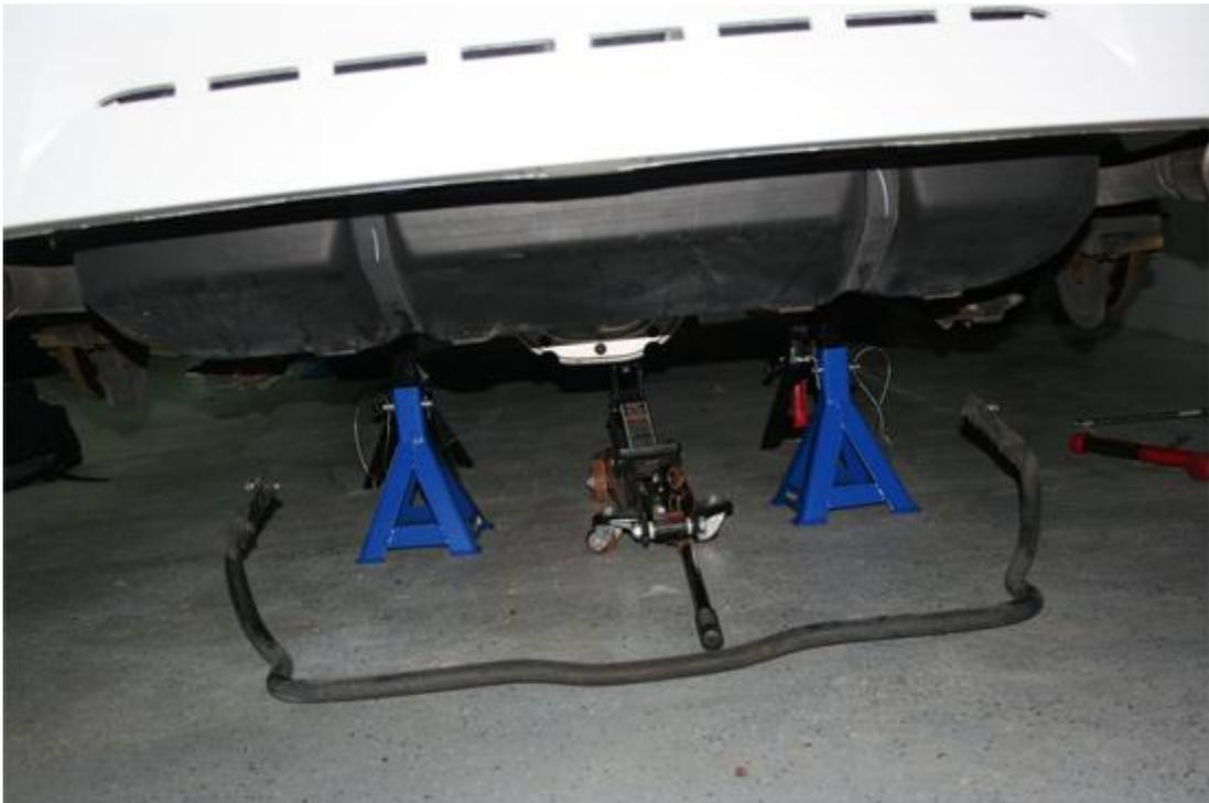
5. Now you will need to move the jack under the control arm and place slight pressure up to the control arm. Then remove the bolt with a 21mm socket and ratchet wrench. A 18mm back up wrench may also be needed.
