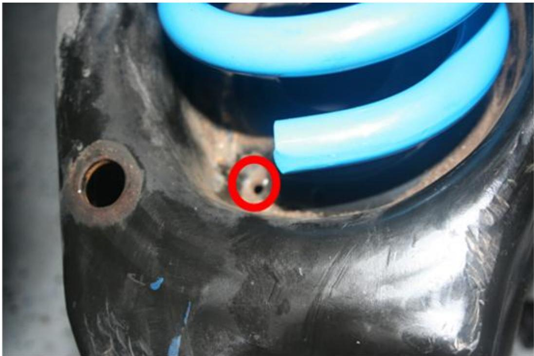
19. Now with the new spring installed jack the control arm back into place and reconnect the three components. Then repeat on the other side. Be sure to get the vehicle aligned after completion.
