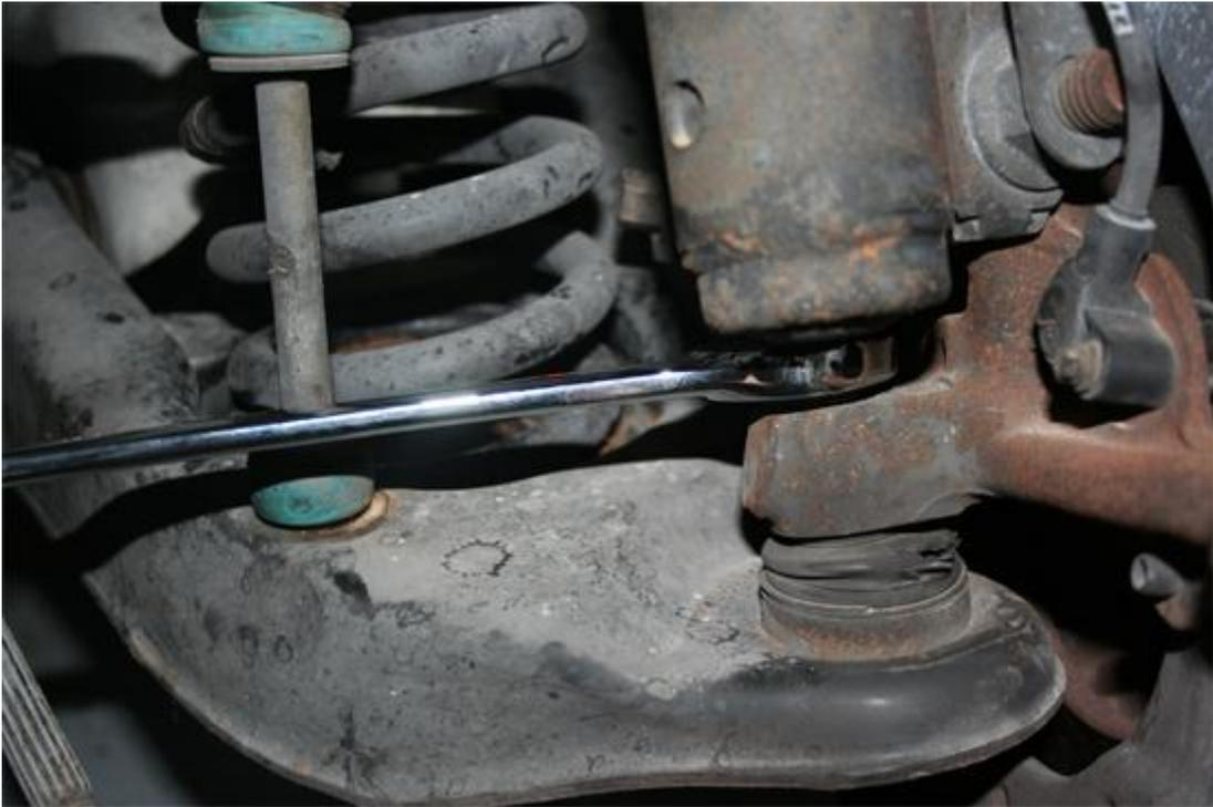
15. I replaced the ball joints also at this time, so I used a pickle fork to separate the ball joint from the spindle. However you may use you mallet again to break this joint. The use of a pickle fork does require the replace of the ball joints
