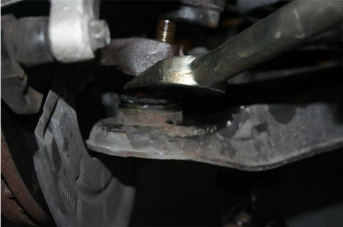
16. Now with these items removed and separated lower the jack to release tension off of the spring. Then use your foot for a little extra clearance and remove the stock spring.
