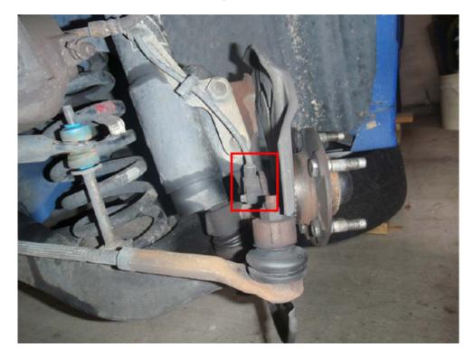
9. Now that all the front steering and suspension components have been detached, the next thing you want to do is SLOWLY lower the jack still holding the A-arm, until it no longer supports the A-arm. At this point, you should be able to pry your coil spring out of its place using a pry bar, and set it aside.
