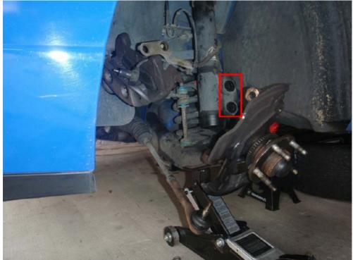
7. Continue with the driver's side, and disconnect the sway bar end link nut. This nut is also 15mm in size but you will need a deep socket. If you just remove the top nut and top bushing, that is enough.
