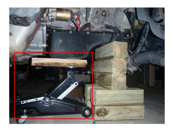
15. After you are sure the jack is in the correct position, use a ratchet with extensions and a 22mm deep socket to remove the motor mount nut from each side of the car. The weight of the motor will keep it secured on the K-member with these nuts removed.
