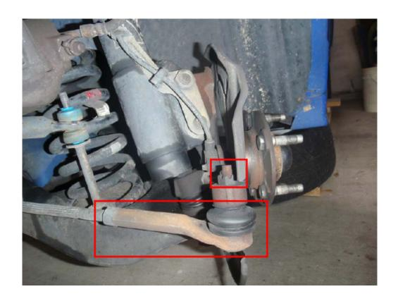
6. After this, you are ready to disconnect the strut. Place the jack under the A-arm again and raise the jack only until it puts pressure on the A-arm. Then loosen the bolts that attach the strut to the spindle. First, remove the nut that holds the ABS bracket in place using a 15/16" wrench. Then, using two 13/16" ratchet/socket combinations or one socket and one box end wrench, loosen the two bolts and remove them.
