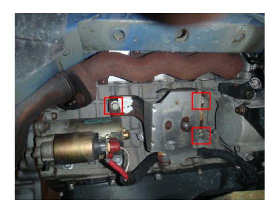
23. Now you're ready to remove the stock manifolds. Using a 13mm deep socket and various extensions, you can remove all the nuts holding the manifolds in place. There are 8 bolts per side and some of the nuts may be stuck to the bolt such that the bolt comes out of the block with the nut. This is ok – do not worry about it. The driver's side manifold also has the EGR tube attached to it. Remove this by loosening the nut with a large adjustable wrench.
