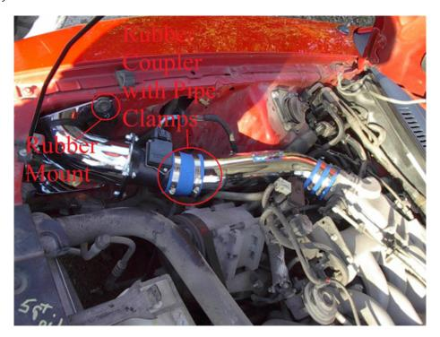
18. Finally, reattach all of your wires to the intake, and check all of your bolts/screws.
