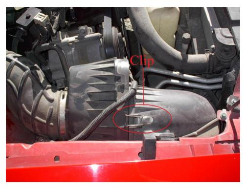
3. Remove the only bolt holding the stock air intake in place. This bolt can be removed with your 8mm ratchet. Save the bolt, for it will be used later in the installation.
