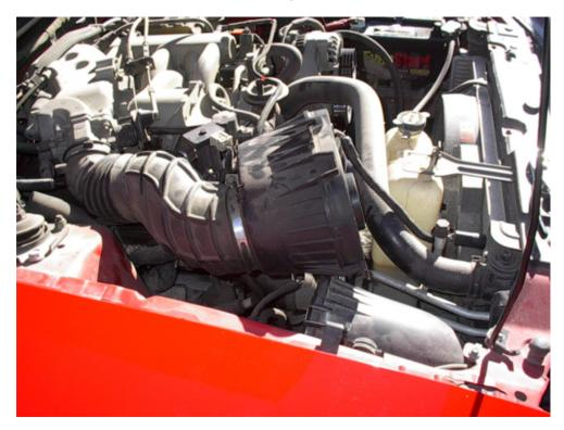
5. Remove the intake snorkel from the fender. It will pull out diagonally from the engine compartment.
