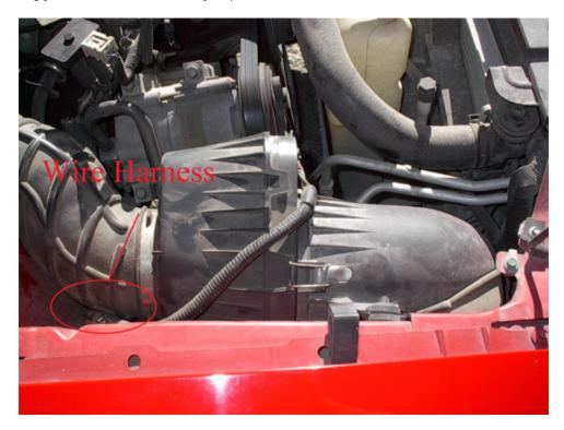
2. Undo both clips on the air filter housing. The first one is visible right on top, but the second is just around to the right of the clip shown.
