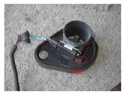
14. Fit the elbow pipe on to the airflow sensor with the 4 10mm bolts and nuts provided. Use your 10mm socket, ratchet, and wrench to tighten the bolts and nuts. Be careful not to over tighten the bolts, for some sensors and plastic and break easily.
