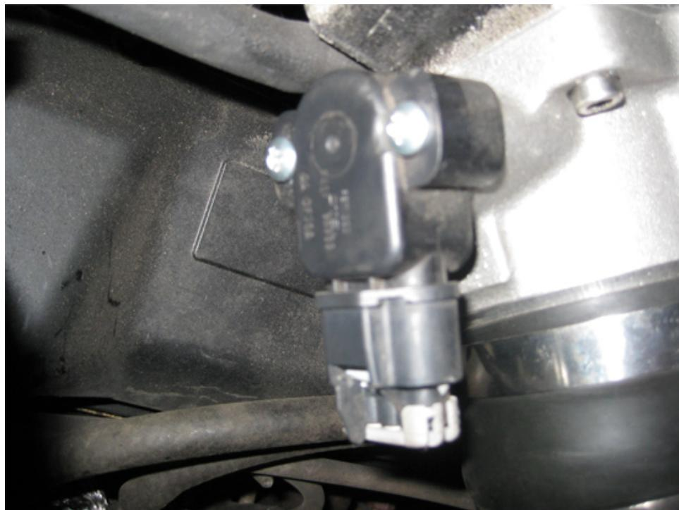
4. Disconnect the throttle cable and auxiliary return cable. The auxiliary return cable pops off with pressure and the throttle cable has a space in the bottom where it can be slid off easily.
