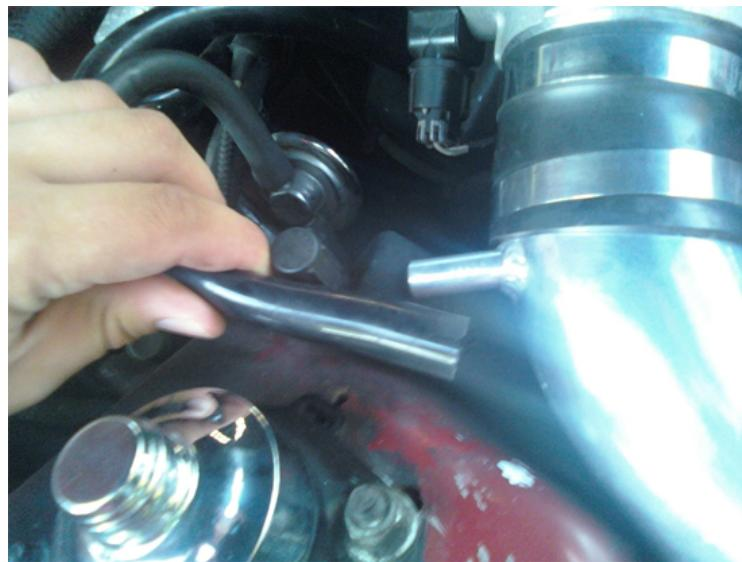
3. Disconnect the Throttle Position Sensor, located on the left side of the throttle body, by removing the two (2) screws on the top and bottom of the sensor.
