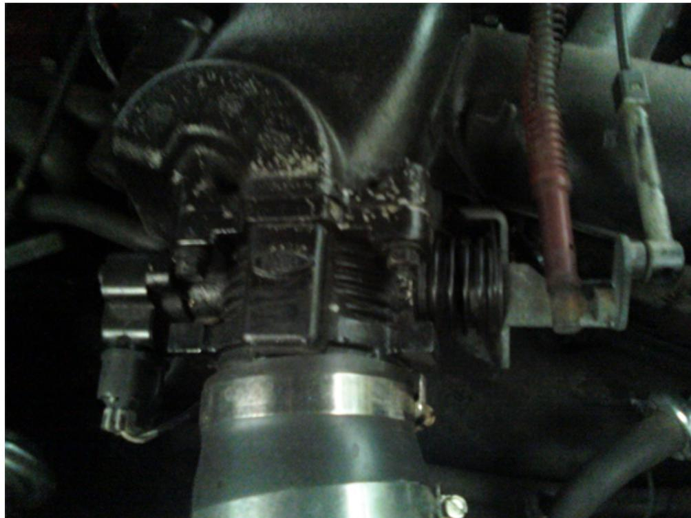
5. Unbolt the four (4) nuts holding the old throttle body.
