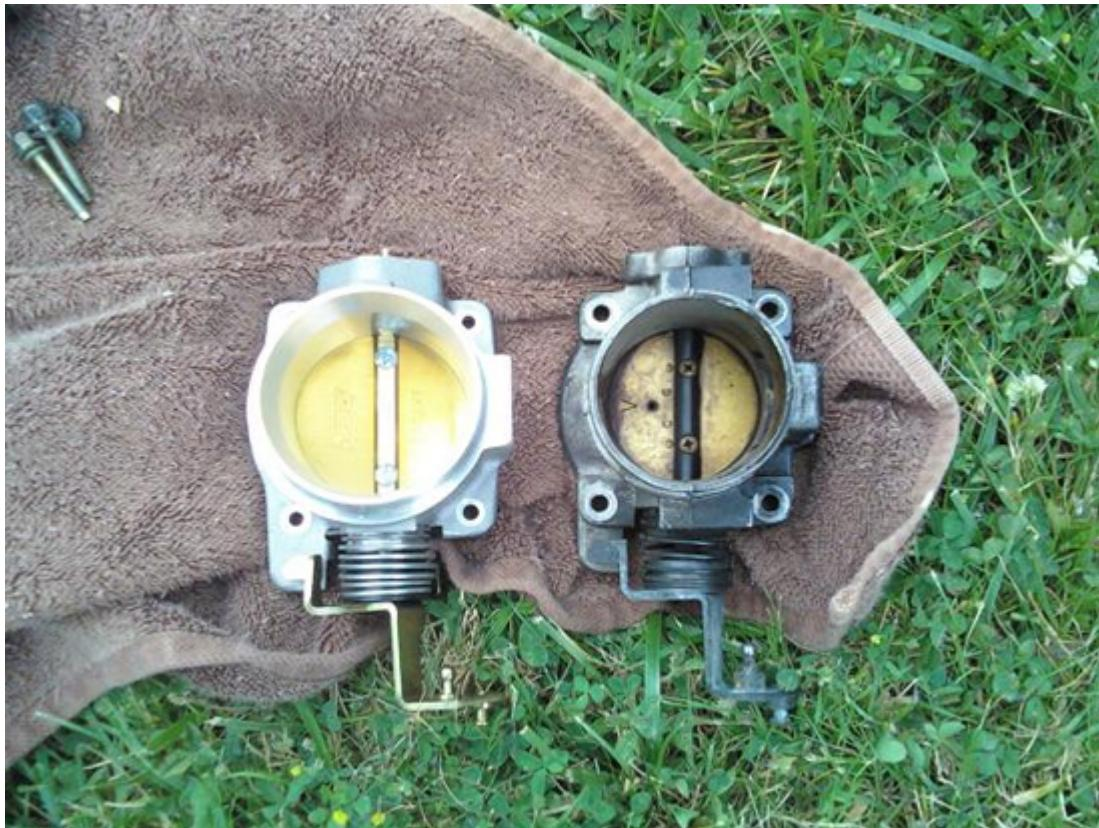
7. After removing the old throttle body, gently clear any debris from where the throttle body was contacting the intake manifold. DO NOT clean inside the intake manifold unless there is a large clump of debris that you know shouldn't be there.
