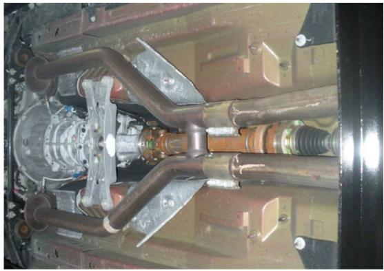
3. Unplug all the oxygen sensors from the stock h-pipe. There will be 3, 1 in each of the catalytic converters and 1 just aft of the passenger side exhaust manifold. Disconnect the O2 sensors from the wiring connectors first so that you do not twist the wiring and possibly cause damage when disconnecting the sensors.
