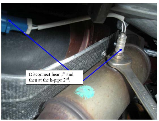
4. Separate the piping connecting the cat-back system to the h-pipe by loosening the 2 nuts on each of the stock band clamps. Pry the locking tabs up with a small flathead screwdriver while sliding the clamp towards the rear of the car.
