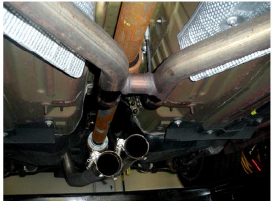
5. Unbolt the stock h-pipe from the exhaust manifold collectors and remove the hpipe from the car. Unbolt the H-pipe from these locations.
