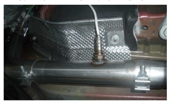
9. Install crossover pipe and position band clamps over connections and re-install the over axle pipes to the crossover pipes at this time.
