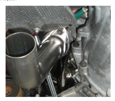
8. Install Catalytic converter/delete pipes to inlet pipes, but do not tighten down the band clamps. Make sure that the O2 sensors are facing up, otherwise you will stretch the wiring and could possibly cause damage during installation.
