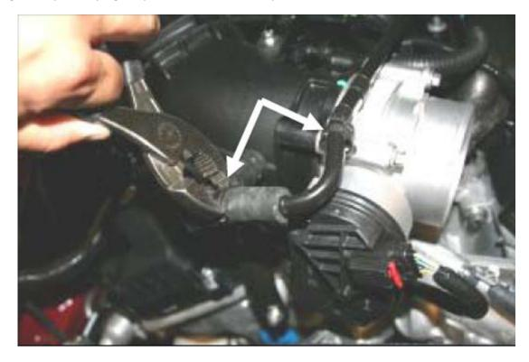
3. Remove the four bolts that secure the throttle body to the intake and set it aside. They will not be reused.
