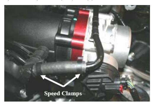
6. Reinstall the intake tube, tighten the two hose clamps, and reconnect the breather line or lines. Reconnect the negative battery cable.
