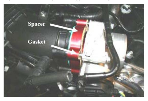
5. Remove the factory breather hose and spring clamps, and replace them with the supplied Breather hose and Speed clamps. Retorque the throttle body bolts in an "X" pattern, to Factory specs.
