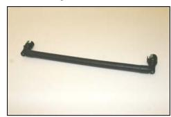
**18.** Install the 3/8"x12" hose (#8) onto the factory breather ends as shown.
