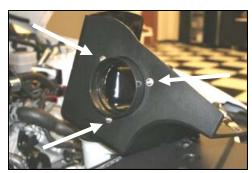
**8.** Install the air filter adapter (#6) into the Cool **Air D**am (#7) as shown, using 3 button head bolts (#10) and <sup>1</sup>/<sub>4</sub>" flat washers (#11).
