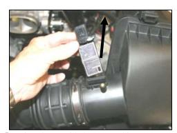
**5.** Using the provided #20 torx bit, remove two screws and the mass air sensor from the factory airbox lid. Note the direction of the sensor for proper re-installation later. (Save the mass air sensor for re-installation in step #13, the factory screws will not be re-used).
