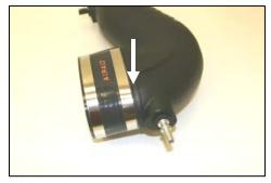
**14.** Install the oval coupler (#4) with two #72 hose clamps (#13). Tighten <u>only</u> the clamp closest to the aluminum fitting. (*Hint: For a clean look, locate the hose clamp tightening screws under the tube*)!
