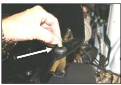
7. Install the provided grommet (#15), with the groove at the top, into the Cool Air Dam (CAD) hole, as shown. Next slide the aluminum sleeve (#16), into the center of the grommet.
