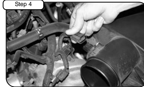
Disconnect MAF sensor harness.
