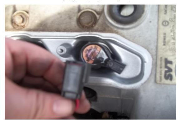
12. Firmly pull upwards on the old coil pack and remove. (mine fought me quite a bit and didn't want to release from the **spark plug**)
