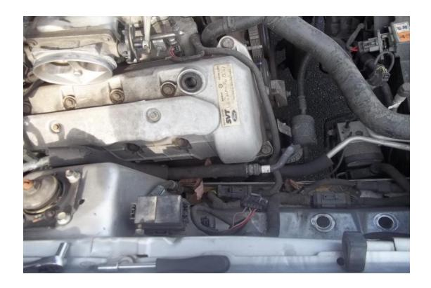
9. Locate the cover over the coil packs and remove the two 10mm bolts.
