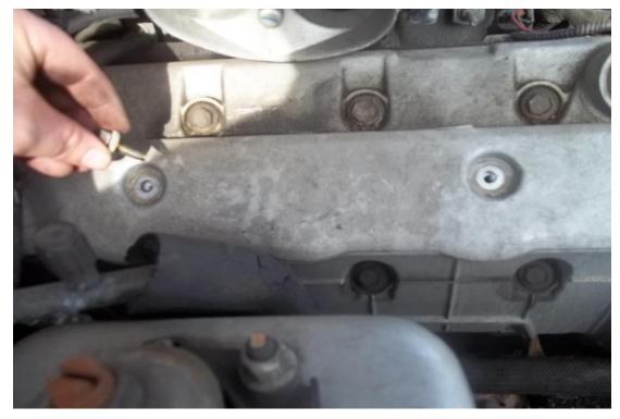
17. Move to the other side and remove the two 10mm bolts.
