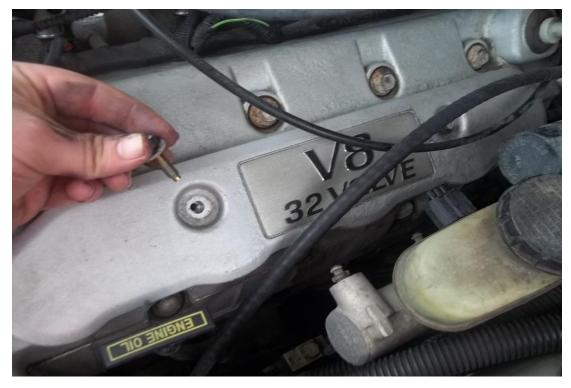
20. Install the air intake, reconnect mass airflow sensor, and the 8mm bolt.
