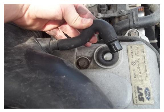
6. Use a flathead screwdriver to loosen the band clamp from the throttle body.
