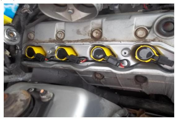
16. Place the cover back over the coil packs and tighten the two 10mm bolts.
