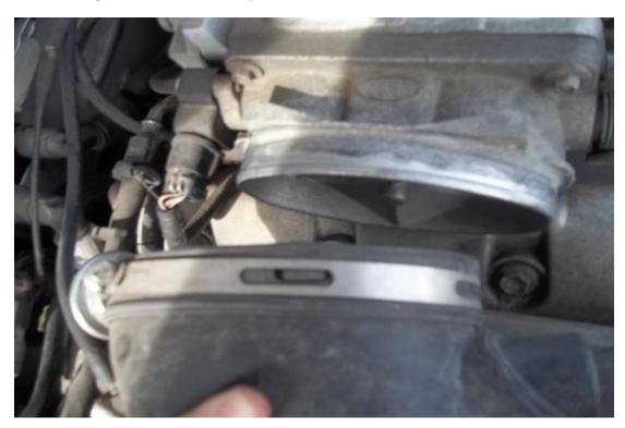
8. Lift the complete air intake system up out of the car, and set aside. (Note there are 2 rubber inserts under the air filter box)
