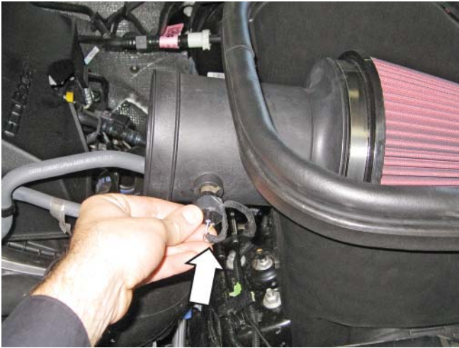
10. Install the two (2) M8 bolts (P/N: W500224-S437) and tighten to 10 Nm.
