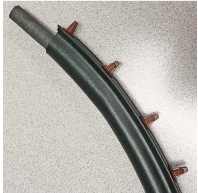
16. Install the air box seal starting in the location shown. You may need to trim your seal to the correct length. ( NOTE: Start the seal at the middle of the inlet tube.)
