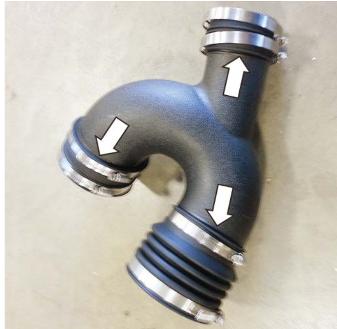
12. Install the clean air tube assembly between the throttle body and the air box. Tighten the clamps to 3 Nm.
