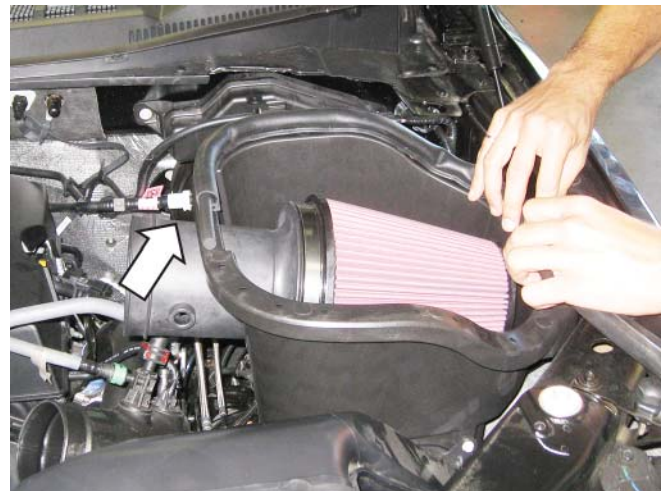
16. Install the air box seal starting in the location shown. You may need to trim your seal to the correct length. ( NOTE: Start the seal at the middle of the inlet tube.)
