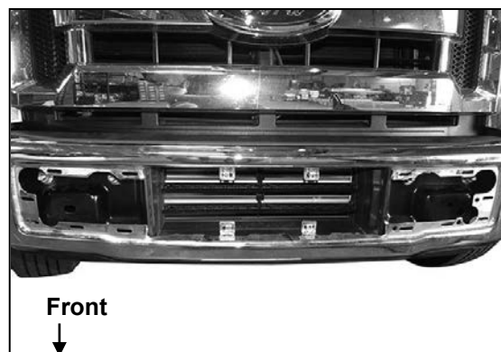
(Fig 2) Remove license plate. From behind bumper, release metal clips attaching plastic bumper pad to the bumper
