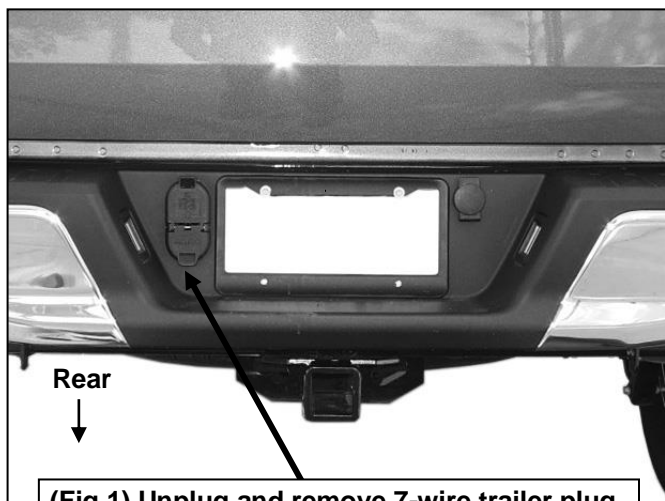
(Fig 1) Unplug and remove 7-wire trailer plug
