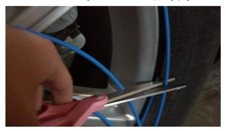
13. Your band, because it may be cut long, may not fit perfectly into the track at first. Go back over the colored band with the application tool pressing the band into place in the opposite direction you had worked before. This will allow for a tight fit.
