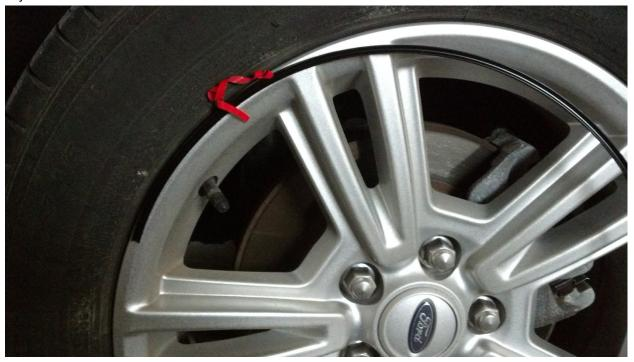
6. When you reach the point where you began sticking the mounting track, cut the mounting track to the correct length using your cutting tool.
