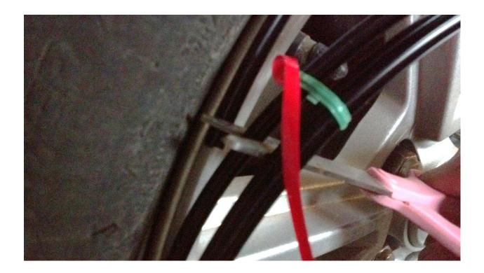
7. If you find that you have cut the track too long, lift up end of track and cut it slightly shorter. It is fine if there is a small gap between the two ends.
