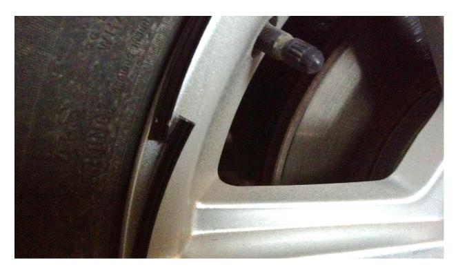
8. Look back over mounting track and adjust until in the desired position. Once this is done, press firmly over entire track.
