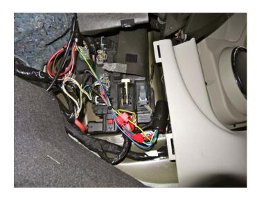
You may wish to insert a small screwdriver into the backside of the connector to unclip the connector cover. This will allow you to separate all the wires and verify the correct wires and pins inside the connector since a few of them look quite similar.
