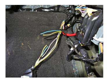
The DRL kit is supplied with white Marrett or Wire-nut joiners, which at this point you can use to join the wires. If you have access to a soldering iron and heat shrink tubing this would be the best method to connect the wires in all electrical projects.
