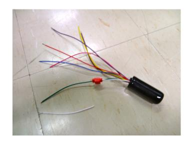
5. Snap and slide the white clip on top of connector C2280F to the left to release the connector from the junction box. Carefully cut the black "wrap tape" from the wire harness and locate the "blue/green" and "yellow/violet" wires. Cut the two wires half way up the wiring harness and strip the ends.
