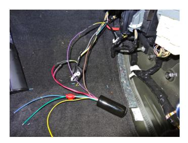
10. Pull down on the white tab to remove connector C2280D from the junction box. Carefully cut the black "wrap tape" from the wire harness and locate the "yellow/gray", the "violet/white" and the "black/white" wires.
