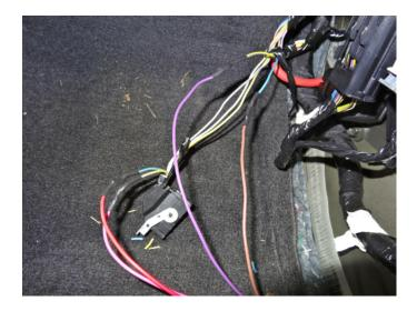
6. Slide a 1.5" length of 3/16" heat tubing over the red wire from the DRL module. Twist the blue/green wire from the connector to the red wire. Solder and then fold over one of the wires. Slide the heat shrink tubing over the solder joint and warm with a heat gun.
