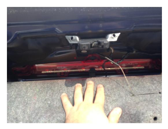
3. Unclip the harness that plugs into the brake light.
