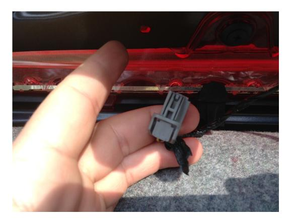
4. Plug in the factory harness into the pulser unit.
