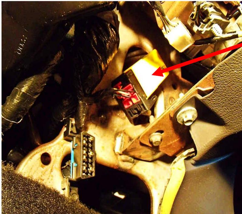
2. Pull the yellow relay unit down towards the OBD II port and out of the bracket holding it in place.
