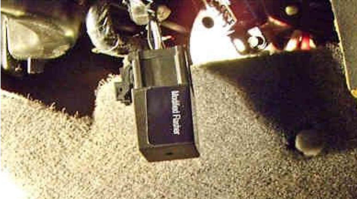
4. Reattach the modified flasher unit to the bracket underneath the dash.
