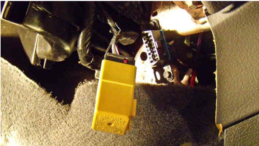
3. Unclip the yellow OEM flasher unit and replace it with the Raxiom Modified Turn Signal Flasher. Be sure to line up the blade connectors in the same manner as the OEM unit.
