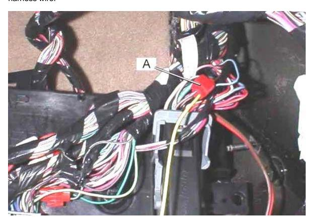
4) Rotate the SJB to expose the connectors on the front of the unit. Referring to the diagram below, find the small, blue connector and make the following connections:
