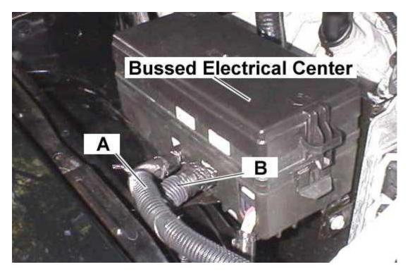
1) Open wire loom "B" (if necessary, remove or carefully cut any electrical tape to increase access to the wires). Locate a RED/YELLOW STRIPE wire. There are two of them -- you can pick whichever is easier to work with. Using a quick-splice, connect the YELLOW module wire to the RED/YELLOW STRIPE wire in the harness.
