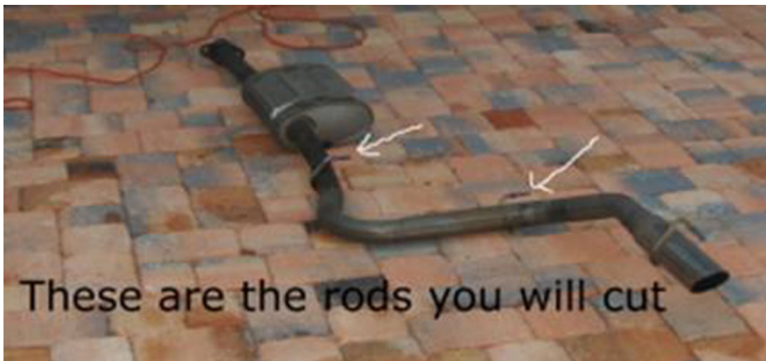
This is the old exhaust which has already been taken out.
