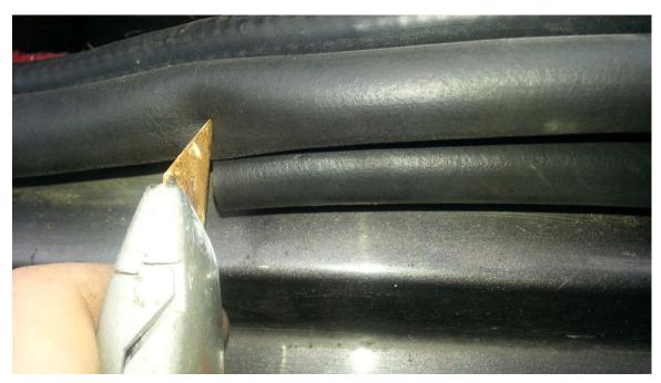
3. Here you can see the small metal tab. Its function is to keep tension on the weatherstripping to keep it clamped on the pinchweld. There are more like it just behind it. You will remove this tab. I was able to pull it out with my fingers.
