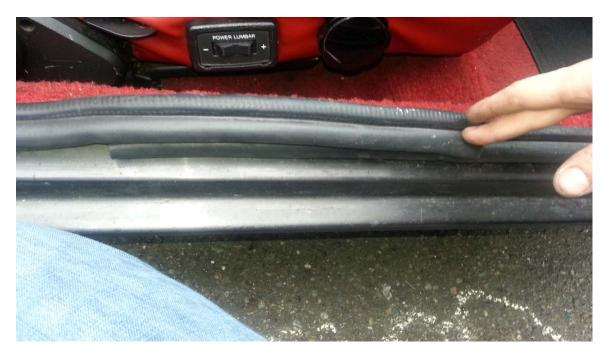
2. Using a razor blade utility knife, cut the outer portion of the weatherstripping. Then cut into the part that seats onto the pinch weld. On both sections of weatherstripping I did, there was a metal tab where I needed to cut.
