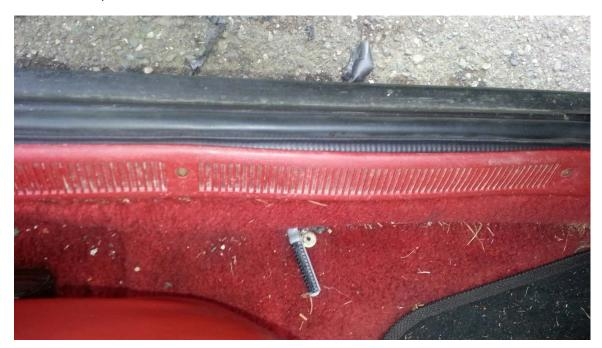
3. Remove the upper trim panel. There are two metal clips holding this in. Pull down slightly on the trim panel, then insert the flat blade screwdriver against the metal clips and push them towards the interior. These clips can be a bit of a pain, but once they release, the panel will pop free.
