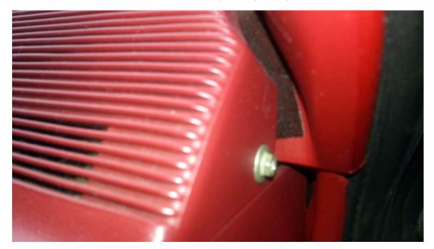
**6.** Remove the side windshield trim panel. There are three screws holding this in. One at the top which was covered by the top trim panel (mine was broken), one in the middle and one at the bottom by the speaker. These are all Phillips head screws of varying length, so label or remember where you removed them from. Once the screws are removed, it takes a little wiggling to get the panel out
