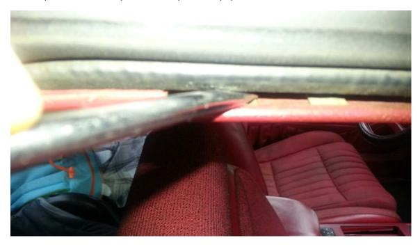
**4.** Remove the upper windshield to headliner moulding. This pops out the same way as the upper trim panel. You do not have to remove the whole thing, but it makes it a lot easier if doing both sides.
