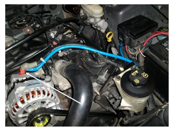
4. Remove the nut from the battery positive side of the solenoid. You will need a 9/16 socket. See photo for location. Fender well next to washer fluid reservoir. You will slide up the case (see arrow below). This will allow you to connect the other end of your PAP wire with fuse box). You will want to connect the shorter end to the fuse box.
