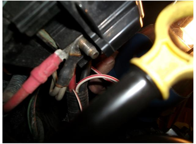
5. Connect and slide fuse box tab back down. Position the PAP fuse box tucked up next to battery box. Use zip ties to neatly strap down the PAP cable.
