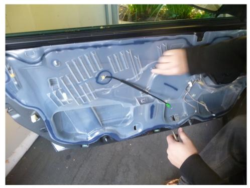
4) Peel back this cover (breaking the silicone bonds with your hands/a tool) on the right side. You'll need to lift the cover over the door lock pin to remove it.
