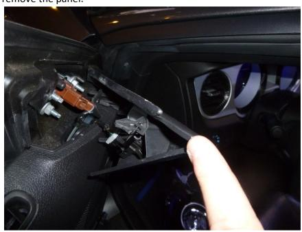
2) Pry up the window controls, again using the pry tool. Disconnect the connector by pressing on the tab and pulling apart
