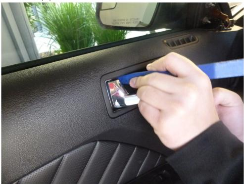
6) Using a pry tool along the outer edges, pop off the speaker cover
