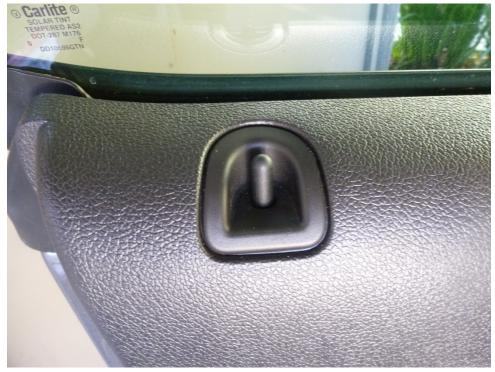
4) Pry up the door trim grip bezel with the pry tool; it is much easier to pry this up when coming through the hole in the grip.
