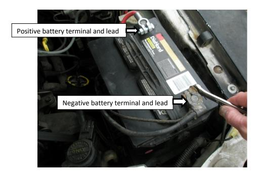
2. Disconnect the positive battery terminal with a ½ inch open end/box end wrench. Using a 10mm socket and ratchet, remove the battery hold down bolt and remove the plastic hold down. Remove the battery from the car.
