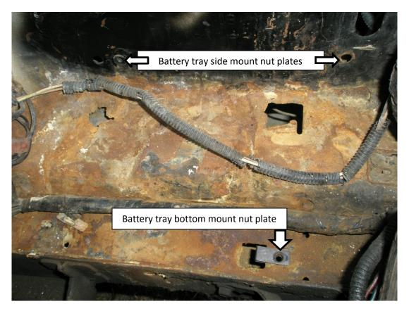
5. Install battery tray side mount bolts using an 8mm socket and 1/4 or 3/8 inch drive ratchet. Leave this bolt loose for alignment of the other mount bolts.
