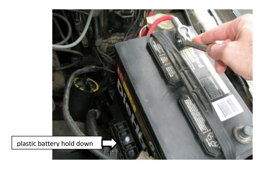
3. Prepare to remove current battery tray from vehicle using an 8mm socket and ratchet for the side mount bolts and a 10mm socket and ratchet for the bottom mount bolt. After hardware is removed, remove the battery tray from the car.
