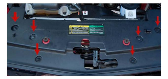
After removing the radiator cover, locate the (8) plastic tabs that hold in the stock grill and remove.
