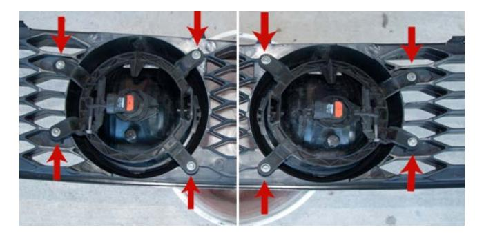
6. Screw the fog lights into your new grill and re-connect the fog lights using your wire extensions as seen in the photo below.
