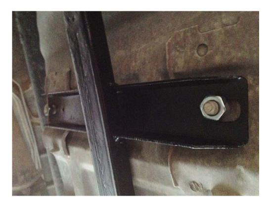
3. Mark the locations on the body and the subframe connector where the front and rear section of the existing subframe meet the subframe connector.
