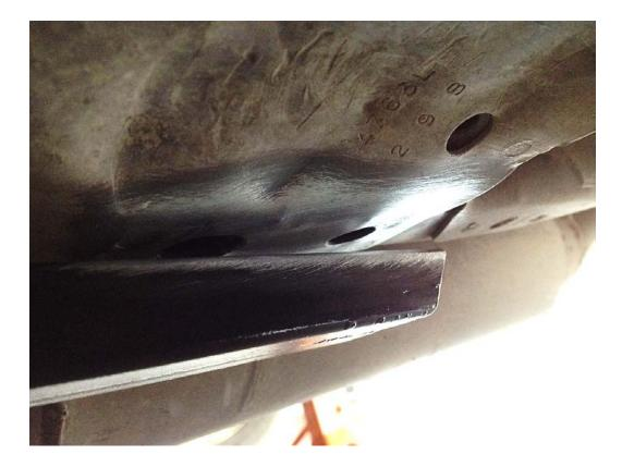
6. Re-install the subframe connector and weld the subframe connector to the existing subframe.
