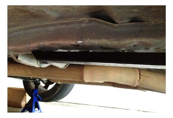
5. Remove the subframe connector and using a wire wheel or sandpaper, remove the paint from the surfaces where the subframe connector meets the existing subframe.
