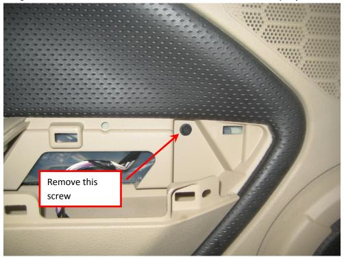
10. There is a friction fit cover in the interior door handle recess that you need to remove. Once again a small but wide flathead screwdriver will work if you do not have panel removal tools.
