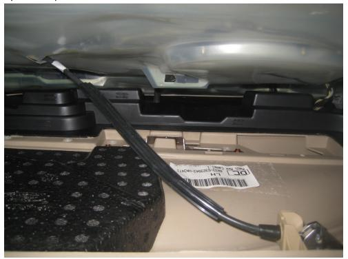
15. Remove the speaker pod by using a 6mm socket on the 3 screws and pull the pod away from the door (there are clips holding it at the screw holes) but don't pull too hard because there is a wiring harness. You do not need to disconnect the wires from the speaker pod.
