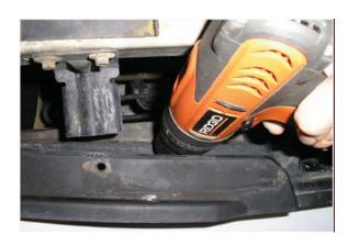
If Re-Installing Pony emblem on billet grille only: Remove the 4 retaining clips on the back of the Pony emblem to release it from the bracket. Clean the back of the emblem and use either silicone, super glue, or 3M tape to apply the emblem to your new billet grille. Be sure to allow time for the adhesvie to set up before driving the vehicle.
