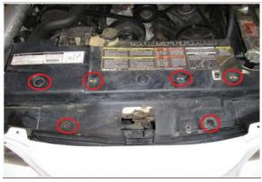
**Step 2:** Remove the Pony emblem and bracket from the vehicle using a Phillips head screwdriver.
