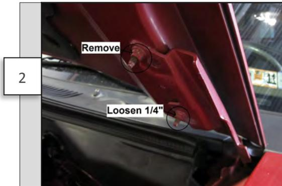
Use a 10mm socket to remove the forward most hood hinge nut. Loosen the rear nut about 1/4" (enough to slide in the upper mounting bracket).
