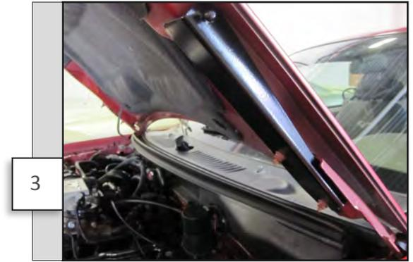
Slide the upper bracket between the rear-most nut and hood hinge and place it over the exposed front stud as shown. Once in place, tighten rear nut and re-install front nut.
