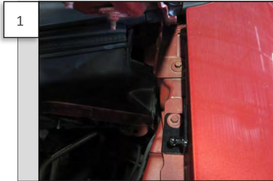
Prop your hood open and remove the 8mm fender bolt shown above (**Do not remove the rear-most bolt that secures the hood hinge**). Place the lower mounting bracket as shown and re-install the fender bolt.
