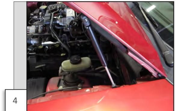
Pop the ends of the strut over the ball mounts on the brackets. Repeat steps 1-4 for drivers side. (**do not slam hood shut yet**) Check bumper/fender alignment by slowly lowering the hood. If okay, remove factory prop rod and enjoy.
