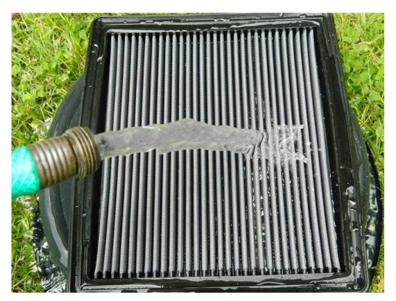
**3.)** Remove water from K&N Filter proceed to hold at (45°) forty five degree angle and allow water to run out you may gently shake excess water out carefully. Allow you're filter to naturally air dry, place filter on a two raised surfaces to speed up drying. (DO NOT OIL UNTIL FILTER IS COMPLELY DRY)
