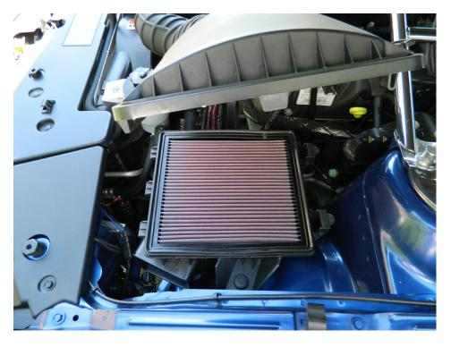
**Notes:** When servicing a K&N filter, take care not to over-oil the element. Besides impeding air flow, excess oil can migrate into the intake system where it can coat electronic sensors such as Mass Air Flow Sensor (MAFS). If any residue or gumming occurs on sensors use only an approved mass air flow sensor cleaner fallowing products directions to prevent any future damage.
