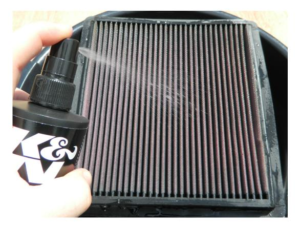
2.) Proceed to rinse off air filter with a cold low pressure water source applied directly to the clean surface of the filter. Repeat steps one and two if filter is still dirty and not completely white. (REMOVE ALL TRACES OF K&N POWER KLEEN OR PREVOIS OIL TO PREVENT FUTURE DAMAGE TO AIR FILTER.)
