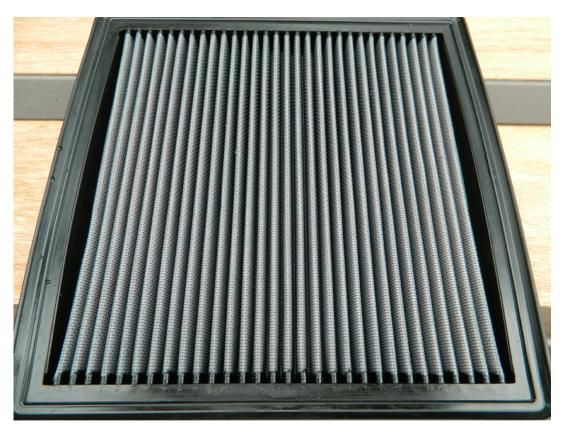
**4.)** When applying K&N Recharge oil make sure to evenly spray along each pleat and crown holding the can 3" inches away from filter surface. Allow oil to wick in completely for approximately twenty minutes. If touch up is required lightly spray those areas until filter is a uniform red color entirely.
