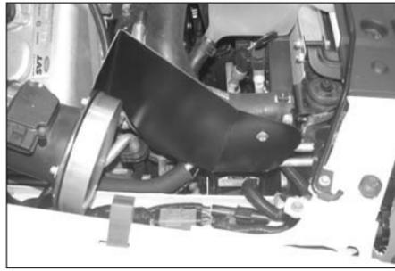
17. Connect the heatshield onto the "L" bracket as shown.
