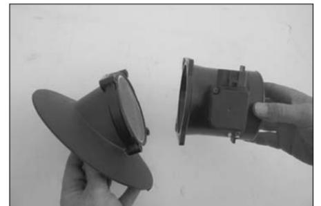
8. Remove the mass air from the air filter housing using a 10mm wrench as shown.
