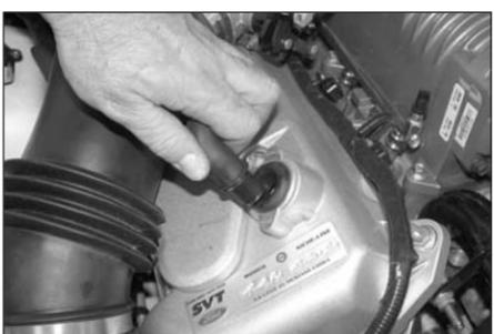
4. Remove crank case vent hose from valve cover as shown.
