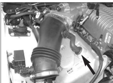
15. Reconnect the intake tube onto the throttle body then reconnect the crank case vent.
