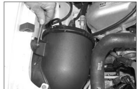
9. Loosen and remove the bolt that retains the air filter assembly onto the vehicle as shown.
