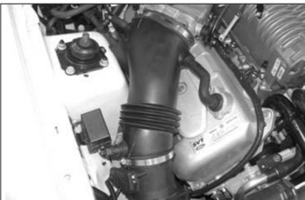
2. Loosen the hose clamps at the throttle body and mass air.
