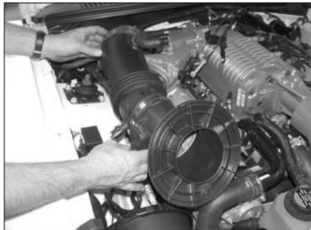
5. Release the intake tube at the throttle body then lift complete intake track up to access the mass air electrical connection.
