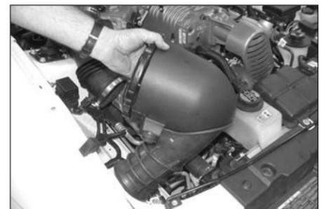
10. Pull the air filter assembly upward and remove from vehicle.
