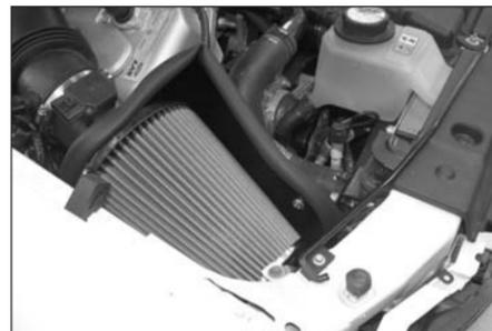
22. Reinstall the mass air assembly onto the intake tube and secure the brackets with the provided sheet metal screw and 6mm bolt onto the "L" bracket.
