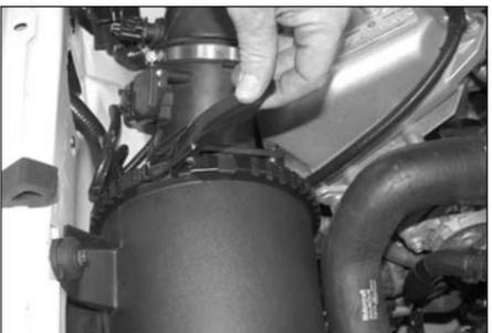
3. Release the filter clam shell clamp as shown.
