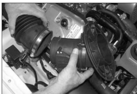
7. Disconnect the mass air from intake tube as shown.
