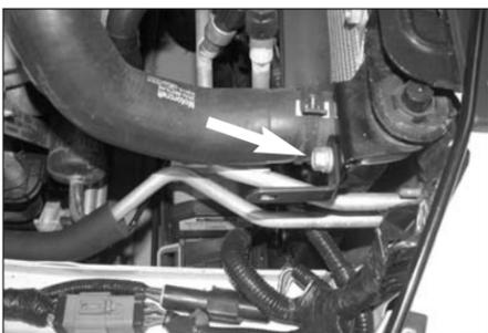
14. Install the provided bracket onto the radiator using the bolt that was removed in the previous step.
