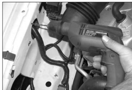
19. Remove the mass air assembly from the vehicle and using a 3/16 drill bit, drill out the marks.
