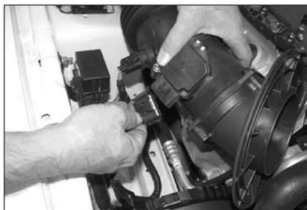
6. Disconnect the mass air electrical connection.
