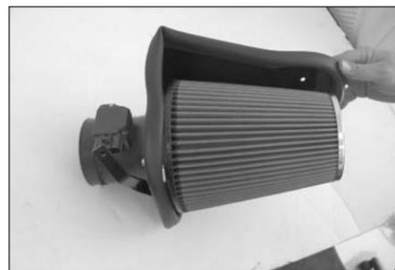
21. Install the filter charger onto the mass air assembly and secure it with the provided hose clamp.
