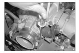
22. Install the provided silicone hose and hose clamps onto the throttle body as shown.
