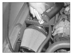
26. Install the K&N Air filter and secure with the provided hose clamp as shown. Adjust intake tube and tighten all clamps completely.
