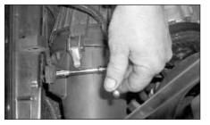
6. Using a 8mm wrench or nut driver, loosen and remove the bolt that secures the air cleaner to the inner fender as shown.
