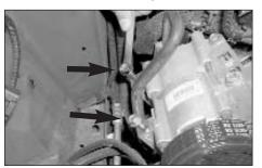
13. Using a 13mm wrench loosen and remove the two lower A/C compressor bolts as shown.
