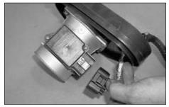
10. Disconnect the mass air sensor electrical connection from the mass air sensor as shown. 14. Using the provided hardware assemble the mass air adapter, heat shield, gaskets, and the mass air sensor as shown using a 10mm wrench or nut driver.
