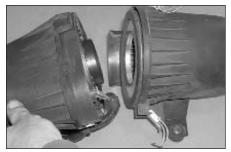
8. Release the over-center clamps on the air cleaner to separate the two halves as shown.
