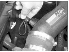
27. On 1999-2000 vehicles reconnect the air temperature sensor electrical connection.
