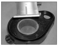
12. Using a 10mm wrench or nut driver loosen and remove the two bolts that secure the mass air sensor, then, remove the mass air sensor from the base plate as shown.
