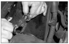
2. Disconnect the secondary mass air sensor electrical connection as shown.
