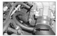
25. Install the provided hose onto the vent on the cam cover, then, reconnect the hose to the 3/8" vent on the K&N intake tube.
