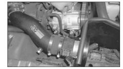
24. Line up the support bracket with the A/C compressor and secure with the original bolts removed in step 13 using a 13mm wrench
