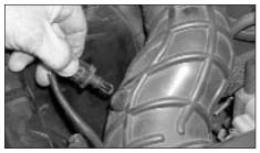
3. On 1999-2000 vehicles remove the air temperature sensor from the rubber intake as shown.
