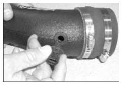
18. On 1999-2000 vehicles install the provided grommet into the hole on the K&N intake tube, then, install the air temperature sensor into the grommet as shown.
