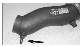
20. Install the 3/8" vent into the K&N intake tube with a 9/16" wrench as shown.
