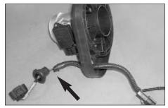
11. Remove the mass air sensor wire harness from the base plate as shown.
