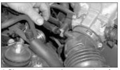
4. Disconnect the crank case vent hose from the rubber intake as shown.
