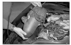
7. Pull firmly upwards to release the air cleaner from the factory grommets, then remove the air cleaner as shown. **Note: K&N recommends that customers do not discard factory air intake.**
