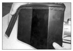
16. Install the provided trim seal onto the heat shield assembly as shown. Trim excess if necessary using side cutters.
