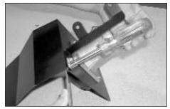
15. Using the provided hardware, assemble the support bracket onto the heat shield using a 10mm wrench as shown.
