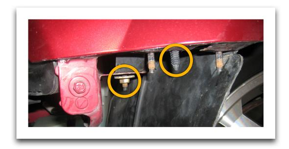
With the bracket replaced now insert the plastic fastener and put on the 10mm nut. Now reinstall the bumper by repeating these steps in reverse.
