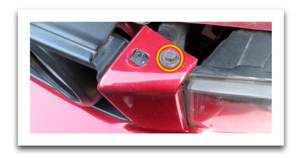
6. You may now lift up slightly to get the top of the bumper off of the plastic hooks at the top. Pull out just enough to gain access to the wiring to the turn signals, fog lights,
