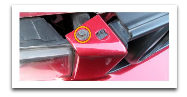
6. You may now lift up slightly to get the top of the bumper off of the plastic hooks at the top. Pull out just enough to gain access to the wiring to the turn signals, fog lights, and headlights. To disconnect the lights they either turn and pull out the bulb or separate the connector.
