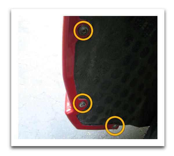
2. Remove the four 6mm hex bolt fasteners under the front bumper that attach the bumper to the splash guard  $\,$
