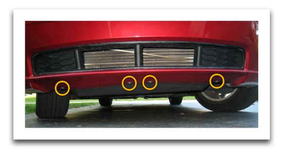
3. Pull back the plastic guard inside the wheel well and use a socket and extender to reach up and remove the two 10mm nuts on each side of the bumper. Pull the sides of the bumper down and slightly out so that the bolts are no longer through the holes in the bumper.
