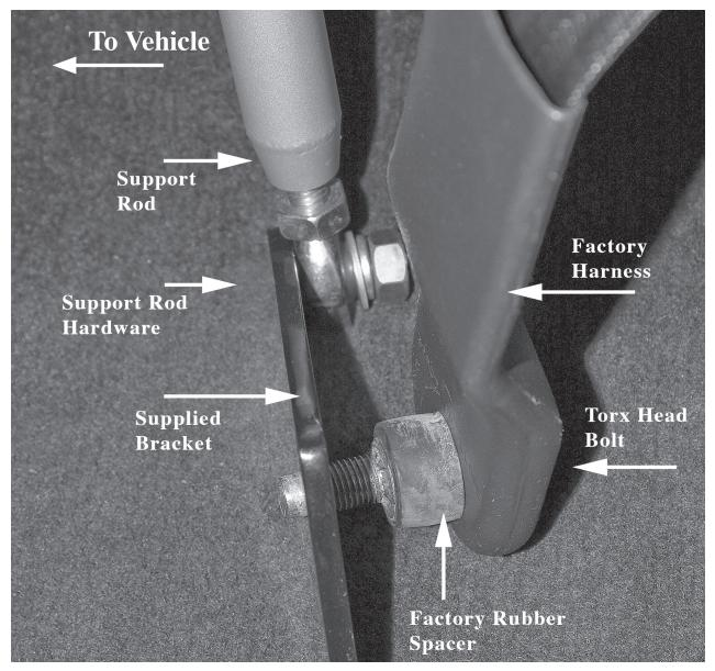
5. Using the supplied bracket, support rod, and hardware. Assemble the bracket as shown. You will then reinstall the stock Torx head bolt into the stock mounting position.
