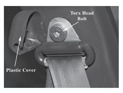
3. Remove the stock retaining washer and bolt from the factory belt. Assemble the hardware as shown and install the harness bar into your vehicle. There might be slight tolerance variations from vehicle to vehicle. Because of this you may need to bend the ends slightly for proper fit. Refer to instruction number 6 for proper stock factory belt routing. At this time you will not fully tighten the nuts.
