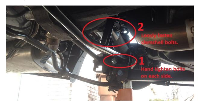
6. Rotate the Swarr bar so the two middle bolt holes are flush on the differential. They should be evenly centered on the differential at this point. Keeping the swarr bar flush to the differential, drill a hole thru the differential on both sides. Be sure to use safety glasses as there will be lots of metal filings falling out. When the two holes are drilled, use the remaining bolts and nuts to hold the two middle mounting points in place.
