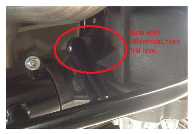
7. Using a 9/16" wrench & a 9/16" socket, extension and ratchet, evenly tighten the clamshell bolts until the clamshell bends about 1/8". Next, tighten the two bolts holding the swarr bar to the differential. Last, tighten the two outside bolts using a 3/4"wrench or socket and ratchet.
