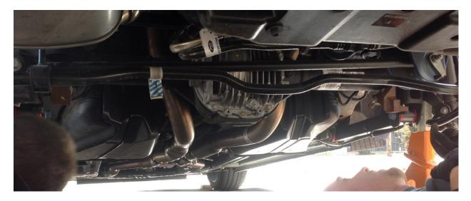
3.Remove the weights on both sides of the axle using a 15mm socket and ratchet. The weights will not be used with the swarr bar installed.
