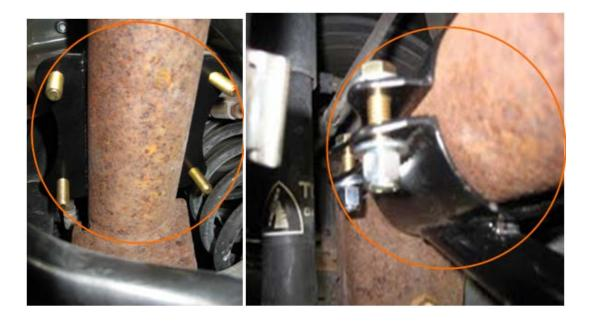
5. Now center the mounting tabs of the Swarr bar to the tabs on the differential housing.
