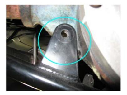
10. After enlarging the holes insert the supplied 3/8 bolts into the tab holes install washers and lock nuts then snug up the bolts ,check the alignment on the axle .
