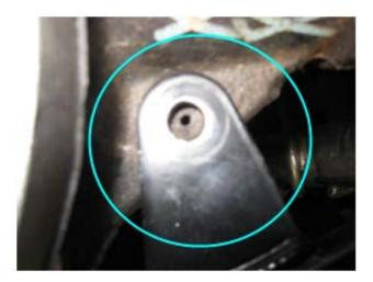
9. Next with the 25/64 drill bit enlarge the holes.
