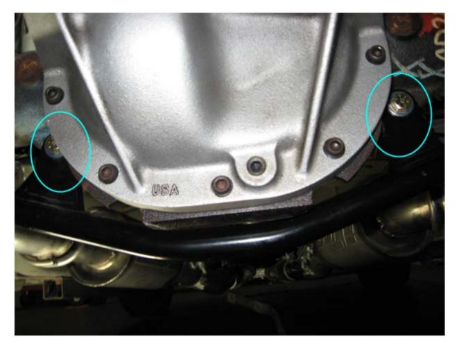
11. Tighten up the tab bolts first using the 3/8 ratchet, 9/16 deep-well socket and 9/16 wrench.
