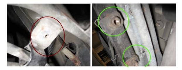
4. Using the supplied 3/8 bolts washers and lock nuts loosely place the Swarr bar on the rear axle.
