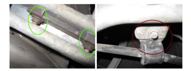
3. Remove the 8 mm bracket bolts then move on to the 15 mm stabilizer bolts; you can now lower the stabilizer bar out of the way.
