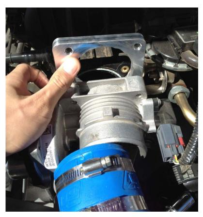
5. Insert the (4) new throttle body bolts into the throttle body and spacer. I started with the top so I do not have to worry about alignment on the bottom where it is hard to see.
