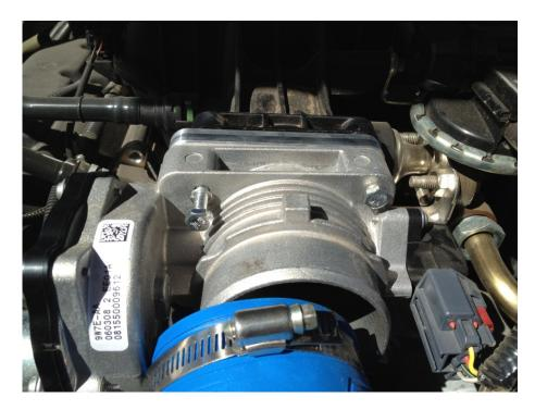
6. Attach the intake onto the throttle body.
