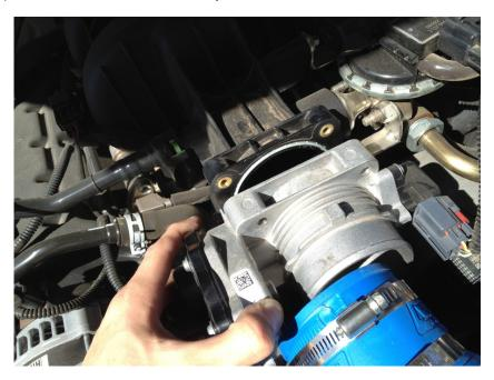
4. Slip the throttle body spacer in between the throttle body and the plenum. Make sure the longer side is facing to the passenger side.
