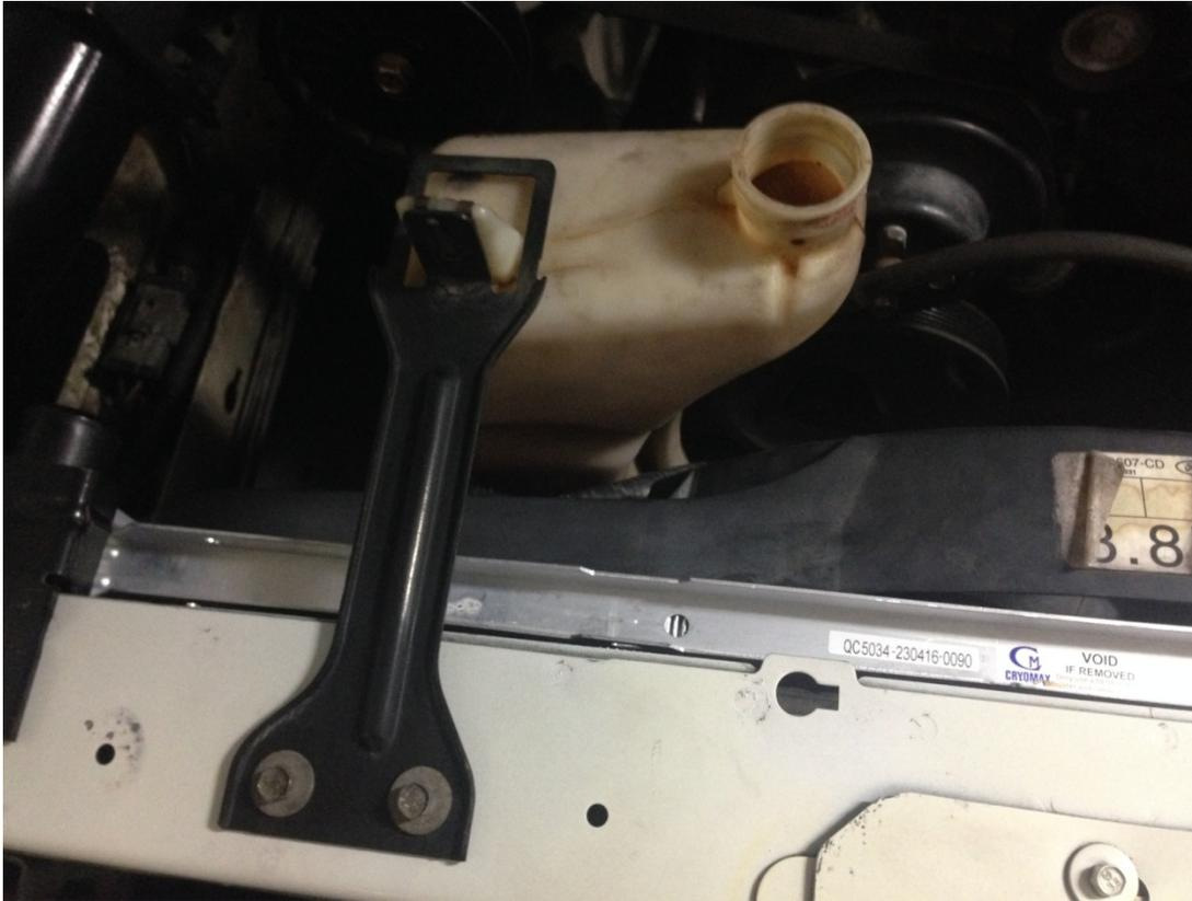
6. Next is the cooling fan which is held in by two 8mm bolts, one on each side and an electrical connection in the middle. (Fan will then lift right out)
