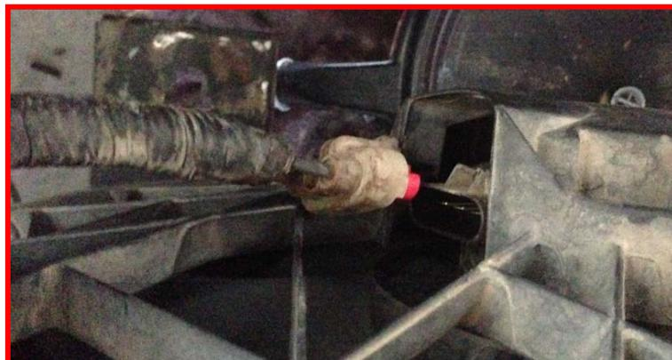
7. Lastly, there are two brackets with a single 8mm bolt holding the radiator in place.
