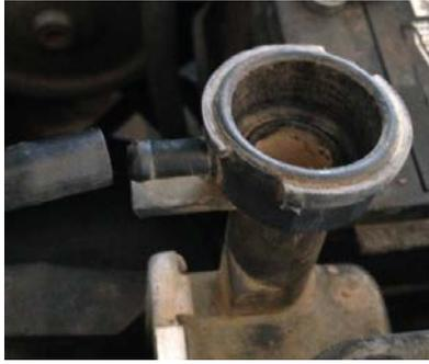
4. Use some large pliers to pull back the clamps on both ends of the upper and lower hoses. Then remove the hoses and place off to the side
