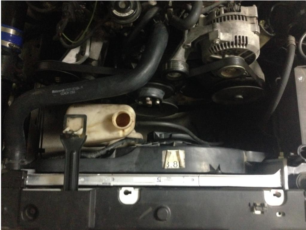
11. Finally refill your coolant with a 50/50 mix green. I recommend having a new radiator cap and 3 to 4 gallons of coolant so you can properly bleed all air out of the system.
