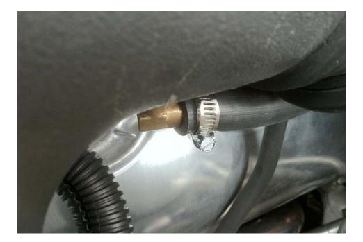
7. Run the hose back to the oil catch can. Cut to length and attach the supplied hose clamp using a flat head screwdriver to tighten. You can also zip tie this line to some other wires for a clean look.
