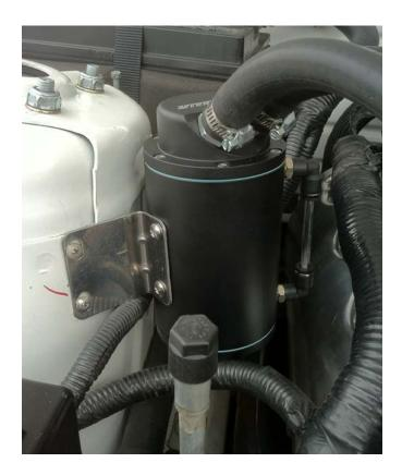
6. Locate the PCV fitting on your cold air intake. Connect the hose to the fitting with the supplied hose clamp and a flat head screwdriver.
