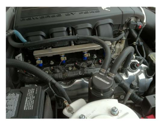
8. Run some more hose from the oil catch can to the PCV valve. Cut to length and attach with the supplied hose clamps, using a flat head screwdriver to tighten. I ran mine to the passenger side PCV valve.
