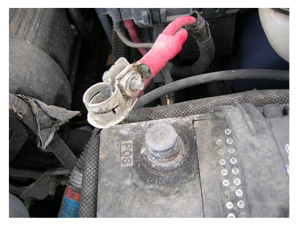
11.) When you are finished filling the coolant reattach the positive battery connection and you are ready to take the car out for a drive. Make sure that you have added enough coolant as air pockets with work their way out after a good drive.
