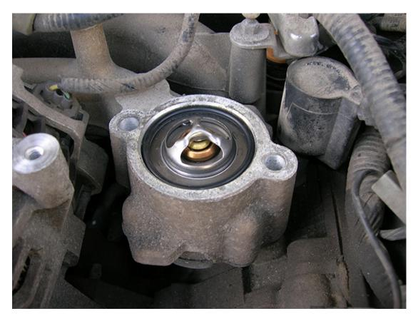
7.) Now get your torque wrench. Set it to 18 ft/lbs or 25 Nm. Put the housing back on and tighten up the bolts.
