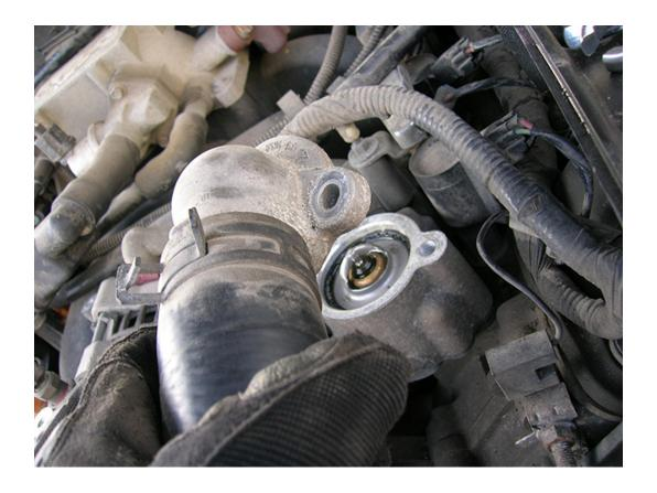
5.) Use a screwdriver to carefully pull the old thermostat out. Be careful not indent the housing. Vice grips may also work well for this step.
