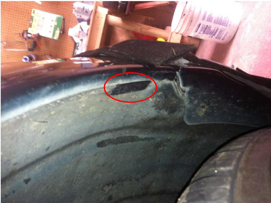
6. Pull the bra up and bend the top tab of the bra around the Velcro strip you just installed. Then bend the remaining two lower tabs around the wheel well and repeat this step on the other side.
