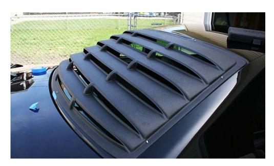
5. Next, carefully remove the nuts and washers from the louver and slowly the louver from the window, leaving the mounting plates stuck with blue tape to the glass. If the plates are moving around on you, use more painters tape to secure each plate individually.
