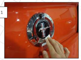
Using the supplied alcohol prep pad, thoroughly wipe down the chrome plated area of the emblem where the cover will adhere.
