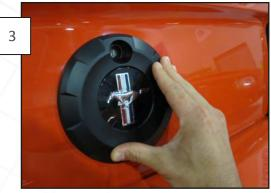
Install the cover over the emblem as shown, making sure it is aligned properly. Once the cover is properly positioned, press down firmly around the edges to fully seat the adhesive tape.
