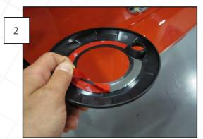
Peel the backing from the adhesive tape by using the supplied tab as shown.
