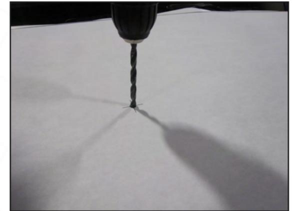
STEP 5 // From the underside of the hood, drill out the front two 1/4" holes to 1/2". Note: If leaving the hood on the car, have a partner hold a shop-vac or similar next to the bit to prevent any metal shavings from landing in the engine bay.
