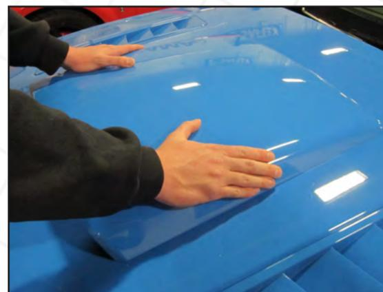
**STEP 10 //** Once the scoop is fully seated, open the hood and install the washers & nuts over the clips studs and tighten with a 7mm socket. Re-install the hood insulation pad removed in Step 1 to complete the installation.
