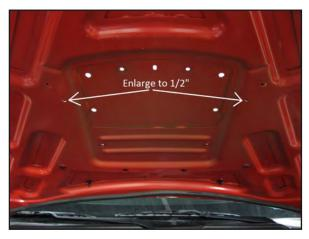
STEP 4A: From the underside of the hood, drill out the front two  $\frac{1}{2}$ " holes to  $\frac{1}{2}$ ".
