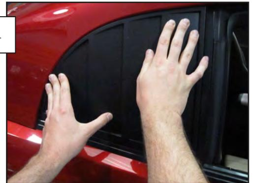
Place the cover on the window, aligning it first with the bottom rear corner and weatherstripping. Once it is properly aligned, press down firmly around the outside edges to fully seat the adhesive. Repeat Steps 1-5 for the opposite side.
