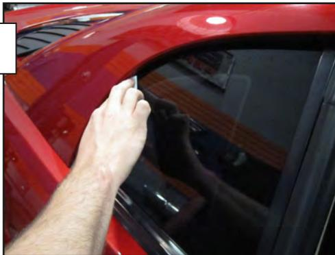
Using the supplied alcohol prep pads, thoroughly clean the outside edges of the quarter window where the adhesive will attach.
