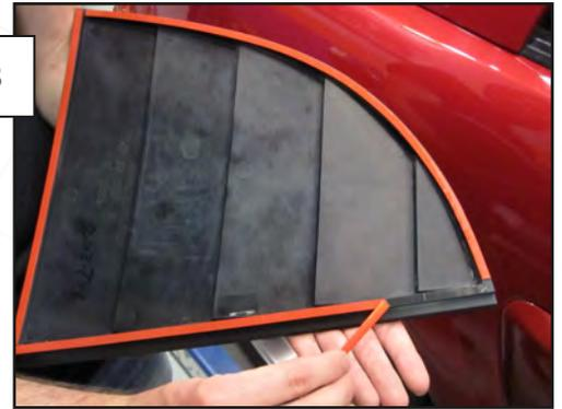
Peel the backing from the 3M Adhesive as shown below.
