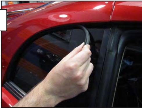
There is a small piece of rubber weatherstripping on some 99-04 cars that will have to be removed prior to installation. If it is present on your vehicle, simply start pulling the strip out as shown in the photo below until it comes completely out of the channel. \*\*\*Removing the rubber strip will not cause any issues, as the negative space will be taken up by the window cover and prevent any possible leaks\*\*\*
