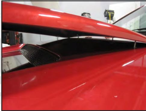
Place the scoop on the hood aligning the rear studs first. Don't fully press down on the scoop until all studs are properly located and the scoop is in its desired location. Once it is properly aligned, move around the edges and firmly press down to fully seat the adhesive.
