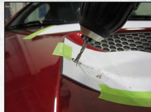
Center punch the 7 holes and drill up to a 3/8" hole. (It may help to step up gradually to 3/8" by using 3/16" then 1/4" bits) When finished, remove the drill templates and clean up any leftover fiberglass shavings using a Shop Vac.
