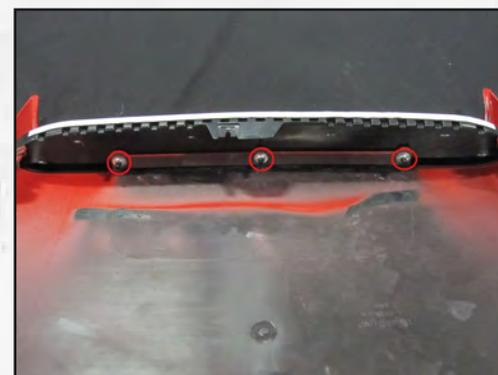
Install the honeycomb insert into the scoop and secure it with the 3 provided locking rings.
