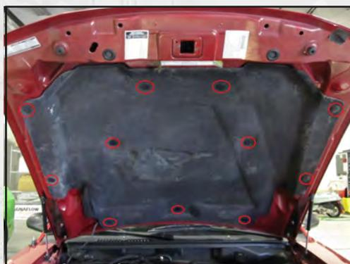
Open the hood and remove the 11 plastic retaining pins securing the hood insulation pad. A trim removal tool works best for this job, but a flat head screwdriver can be used. Once all of the clips are removed, set the insulation pad aside.
