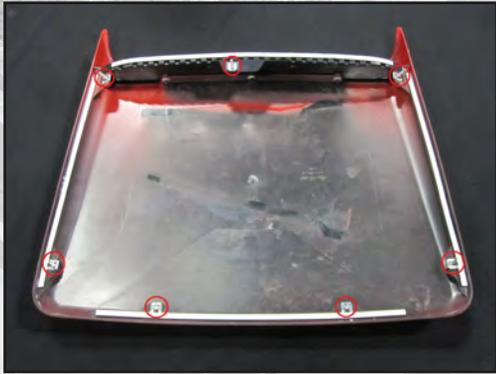
Install the 7 U-tabs/studs onto the designated areas on the scoop.
