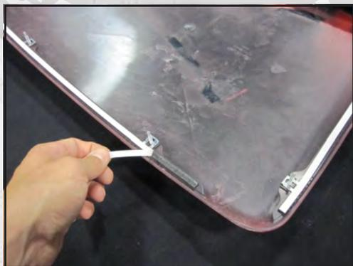
Remove the adhesive foam backing as shown above.
