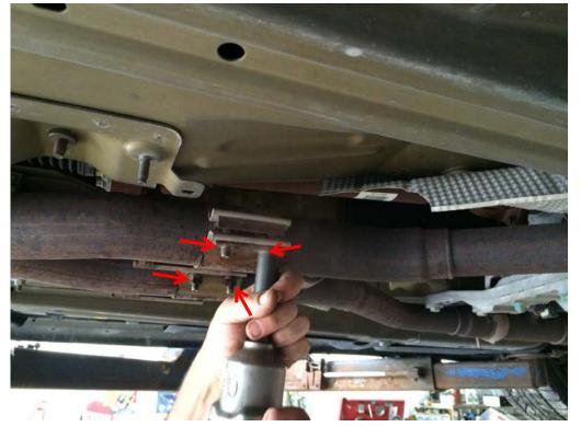
2. Loosen the factory clamp on the Mufflers using the 13mm socket. If clamps/bolts are stiff don't hesitate to use some lubricant to remove them.
