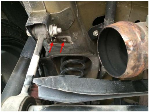
5. Remove the pipe extensions once the mufflers are removed.
