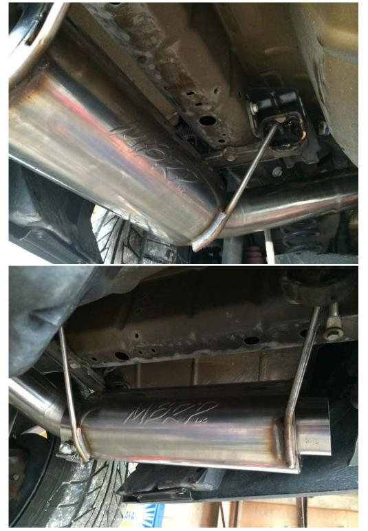
7. Install both extension pipes to the Mid Pipe using the factory clamps. Do not tighten them right away to allow proper fitment with mufflers installed.
